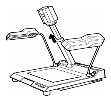
Figure 2-9. Extend the Camera Arm
