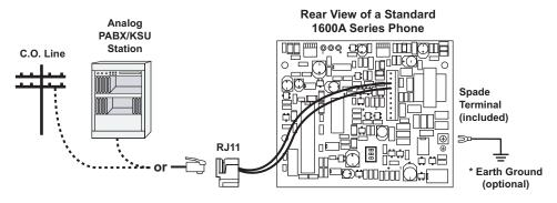
B. 1600A Series Phone with EWP Rear View of a 1600A **Series EWP Phone** Analog PABX/KŠU Station C.O. Line Gel-Filled **Butt Connectors** Spade (included) Terminal (included) \* Earth Ground (optional) Green
