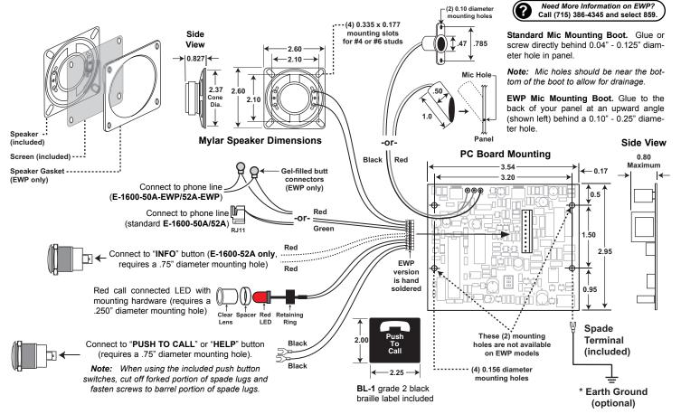
**Important:** If installing the **EWP** version outdoors, apply non-corrosive silicone (included with **EWP** version only) to back side of LED and push button switches after making all connections and testing. Completely encapsulate all exposed switch connections (screw terminals, stripped wire) and bare wire connections.
