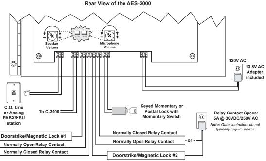
Once the AES-2000 is secured to the wall, the unit can be connected to the building wiring as described below.
