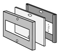
6. Making sure to align all holes, use (2) # 10 Torx head screws (included) to mount the name directory to the surface as shown below.
