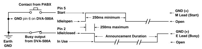
2. Type 5 E & M, wink start. Set dip switches to protocol "B" (Sw 1 - OFF, Sw 2 - ON).
