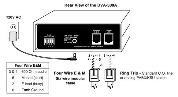
Wire the **DVA-500A** with either or both the 4 wire E&M jack and/or the 2 wire ring trip jack as shown above. When using the 4 wire E&M, the ring trip interface may be used for remote programming. The E&M functions will resume when programming is finished.
