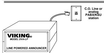
**Power:** Telephone line powered (24V DC @ 20 mA loop current minimum)
