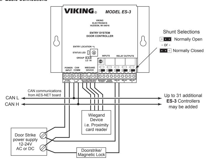
A basic door access controlled entry point is wired as shown above. The **ES-3** may share power with the attached door strike or magnetic lock if the Voltage is between 12-24 Volts and an additional 300 mA of current is available.
