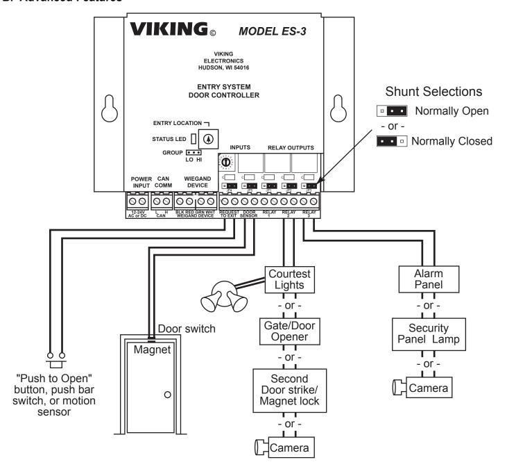
The **ES-3** can be wired with either a normally open or a normally closed Door Sensor switch by setting the shunt located directly behind the Door Sensor screw terminals to either Normally Open (NO), or Normally Closed (NC).
