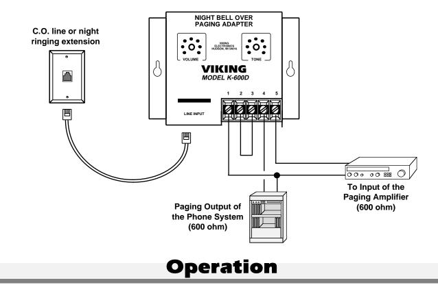
Upon detecting standard AC ring voltage on the **LINE INPUT** jack, the **K-600D** will produce a 600 ohm warble tone in cadence with the ring signal. In addition, the normally open contacts will close and the normally closed contact will open.
