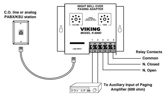
B. Sharing the Paging Amplifier Input with a Phone System Output
