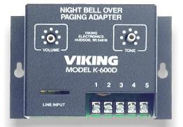
The **K-600D** eliminates the installation of multiple bells, relays and power supplies, whenever night bells, loud ringing or emergency tones are required. The **K-600D** provides an existing paging amplifier with a pleasant electronic warble tone each time it receives ring voltage from a C.O. line or analog PABX/KSU extension.
