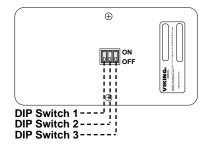
DIP switches 1 and 2 allow the **MOH-2L** to work with varying telephone lines. If the **MOH-2L** does not hold the call that's been placed on hold, the loop current provided by your phone company is probably too low. To compensate for this, set the corresponding dip switch to the ON position.
