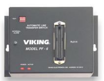
With the **PF-6A**, you will continue to receive your calls, during phone system and power outages. The **PF-6A** bypass unit connects 6 preassigned single line station phones directly to the C.O. trunks you have assigned. A built in ground start converter permits outbound calls from standard phones.
