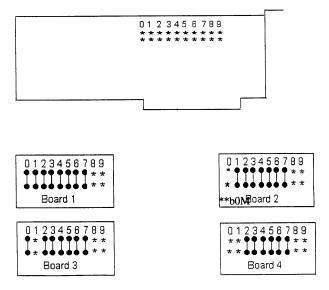
Refer to the above figures to correctly configure the jumpers for each board.
