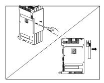
If you are replacing the second module in a two-slot carrier, remove the two #4 screws holding the carrier in place and gently pull the carrier off the modules.
