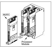
A) Verify that the PARTNER Endeavor processor module is in the center slot of the carrier. In the other slots, from left to right, install the 362EC modules. B) Align the module carefully in the appropriate slot, and push slowly but firmly in the center of the module until the connectors on the module lock into place.
