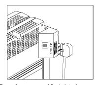
Press the power cord firmly into the power jack on the carrier. Plug the other end of the power cord into a properly grounded three-prong wall outlet not controlled by a switch.
