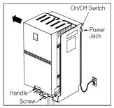
**1** A) Move the carrier's On/Off switch to "Off," and unplug the power cord from the wall outlet. B) To remove the cover, loosen the screw on lower front of the cover. C) Place one hand on the handle on the bottom front of the cover, and place your other hand on the top of the cover. Gently pull the cover up and away from the carrier.
