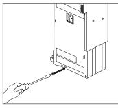
Insert the 3 1/2" #8 screw into the bottom of the modules. Tighten it until the mounting tracks of the PARTNER Endeavor processor module are flush against the wall with a 3/8" (1 cm.) gap between the wall and the rest of the PARTNER Endeavor processor module. Do not overtighten, the modules will warp.
