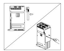
Attach the 2-Slot carrier to the top right side  $\mathbf{6}$  of the two modules:
