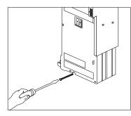
**A)** Remove the #8 sheet metal screw from the bottom of the wall-mounted module or modules.
