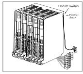
A) Plug the power cord into a properly grounded three-prong wall outlet not controlled by a switch. B) Power up the control unit by moving the On/Off switch to the "On" position.
