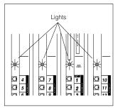
Check the green lights on the fronts of the modules. If a single light is out, power down the carrier, then power up the carrier. If multiple lights are out, power down the carrier, reseat both modules, then power up the carrier. If the lights are still out, in the Continental U.S., call the hotline at 1-800-721-7071. Outside the Continental U.S., contact your Lucent Technologies Representative or local Authorized Dealer.
