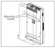
A) Slide the second module off the PARTNER Endeavor processor module and put it aside. B) Slide the 362EC module onto the PARTNER Endeavor processor module, making sure the mounting tracks interlock, as shown in the side view.
