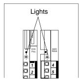
Check the green lights on the fronts of the modules. If a single light is out, power down the carrier, then power up the carrier. If both lights are out, power down the carrier, reseat both modules, then power up the carrier. If the lights are still out, in the Continental U.S., call the hotline at 1-800-721-7071. Outside the Continental U.S., contact your Lucent Technologies Representative or local Authorized Dealer.
