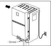
A) To replace the carrier's cover grasp it by its upper edges and hold it squarely over the carrier. B) Place the cover over the modules and make sure it fits firmly in place. If it does not fit, make sure all modules are seated properly. C) Tighten the screw on the lower front of the cover.
