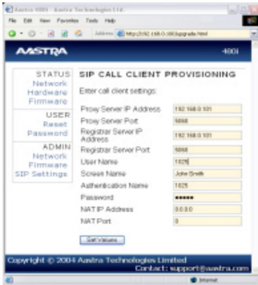
**Note:** At this point modifications performed to the User name, Screen name, Authentication name and Password affect line 1 of the 480i only. Modifications to the other lines should be done through the <mac>.cfg file. The NAT IP Address and NAT Port are currently not supported and will have no effect when set.
