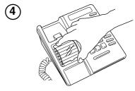
Attach the receiver card and lens (shinyside down) after recording numbers for quick reference.
