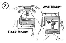
Attach the wedge-shaped base in desk mount or wall mount position†.
