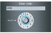
Enter the four-digit security code. If you have entered it correctly, the display changes to the **Disclaimer** screen. If you make a mistake, the system will display "INCORRECT PIN." Re-enter your 4-digit code. You have ten chances to enter the correct code. If all ten are incorrect, turn the ignition to OFF, then back to ON (II) to have ten more chances to enter the correct code.
