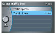
In the example above, only **Traffic Icons** is selected and will show up on the map. To also see **Traffic Speeds** flow on the map, this would need to be turned on by first selecting it and then pushing in on the **Interface Dial** to select it so it appears as below.
