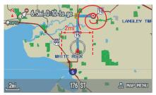
For "Along the route," the system looks in front of you within a corridor width specified by your values for "On Freeways" or "On Surface Street." The system checks a corridor of 1/2 mile on both sides of your current route. For "Around the destination," the system searches outwards in a spiral from the destination. In this case, specific search values are not needed; the matches are displayed in order of distance from destination.
