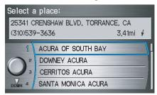
The distance and direction to the destination at the top of the list are shown in the screen. The distance shown is straight line distance (as the crow flies), not driving distance. Say or select the number (1-4) of the desired destination from the list.
