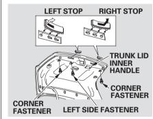
1 a. Determine which back-up light is out (left or right), then open the trunk. aintenanc
