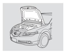
To close the hood, lower it to about a foot (30 cm) above the fender, then press down firmly with your hands. Make sure the hood is securely latched.
