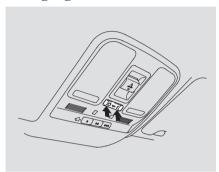
The front ceiling light has a three-position switch; ON, Door Activated, and OFF.
