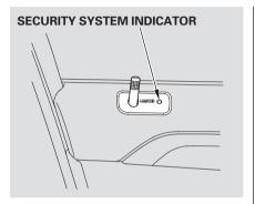
Once the security system is set, opening any door or the hood without using the key or the remote transmitter will cause the system to alarm. It also alarms if the radio is removed from the dashboard or the wiring is cut.
