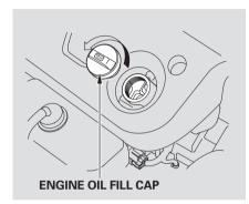
Unscrew and remove the engine oil fill cap on top of the valve cover. Pour in the oil slowly and carefully so you do not spill. Clean up any spills immediately. Spilled oil could damage components in the engine compartment. Install the engine oil fill cap, and tighten it securely. Wait a few minutes, and recheck the oil level (see page 238). Do not fill above the upper mark; you could damage the engine.
