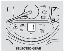
When you move the shift lever from "D" to the Sequential SportShift mode, the display shows the selected gear.
