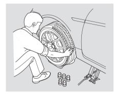
9. Remove the wheel nuts, then remove the flat tire. Handle the wheel nuts carefully; they may be hot from driving. Place the flat tire on the ground with the outside surface facing up.
