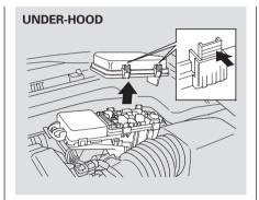
Checking and Replacing Fuses If something electrical in your vehicle stops working, check for a blown fuse first. Determine from the chart on pages 329 and 330, or the diagram on the fuse box lid, which fuses control that device. Check those fuses first, but check all the fuses before deciding that a blown fuse is the cause. Replace any blown fuses, and check if the device works.
