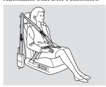
For added protection, the front seat belts are equipped with automatic seat belt tensioners. When activated, the tensioners immediately tighten the belts to help hold the driver and a front passenger in position. The tensioners are designed to activate in any collision severe enough to cause the front airbags to inflate.
