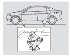
7. Locate the jacking point nearest the tire you need to change. It is pointed to by an arrow molded into the underside of the body. Place the jack under the jacking point. Turn the end bracket clockwise until the top of the jack contacts the jacking point. Make sure the jacking point tab is resting in the jack notch.
