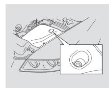
Check the condition of the battery monthly by looking at the test indicator window. The label on the battery explains the test indicator's colors. Check the terminals for corrosion (a white or yellowish powder). To remove it, cover the terminals with a solution of baking soda and water. It will bubble up and turn brown. When this stops, wash it off with plain water. Dry off the battery with a cloth or paper towel. Coat the terminals with grease to help prevent further corrosion.
