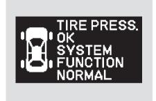
To select the tire pressure monitor, press the INFO button several times with the ignition switch in the ON (II) position.
