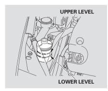
Check the level on the side of the reservoir when the engine is cold, and the engine compartment right-side cover is off (see page 282). The fluid should be between the UPPER LEVEL and LOWER LEVEL. If not, add power steering fluid to the UPPER LEVEL mark.
