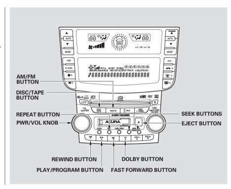
Dolby\* noise reduction turns on when you insert a tape. The indicator will come on in the display. If the tape was not recorded in Dolby, turn it off by pressing the
