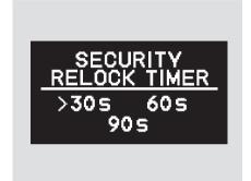
Select the desired relock time by moving the pointer with the INFO (▼) button and enter your selection by pressing the SEL/RESET button.
