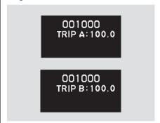
This meter shows the number of miles (U.S.) or kilometers (Canada) driven since you last reset it. There are two trip meters: Trip A and Trip B. Each trip meter works independently, so you can keep track of two different distances. Switch between Trip A and Trip B by pressing the SEL/RESET button.
