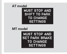
To change the settings, the ignition switch must be in the ON (II) position, and the vehicle must be stopped with the transmission in Park (A/T) or the parking brake set (M/T).
