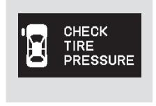
Each tire has its own pressure sensor. If the air pressure of a tire becomes significantly low, the sensor in that tire immediately sends a signal that causes the low tire pressure indicator in the instrument panel to come on. If this happens, you will see which tire is losing pressure on the multi-information display along with a "CHECK TIRE PRESSURE" message.
