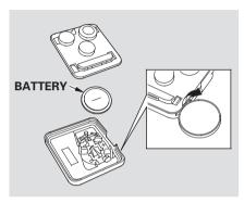
3. Place a cloth on the edge of the keypad, and remove the upper half by carefully prying on the edge with a small flat-tip screwdriver or coin.
