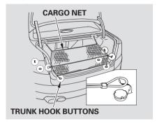
The cargo net can be used to help hold down items stored in the trunk. To use the cargo net, hook it to the buttons on the floor and sides of the trunk. You can use the cargo net in several configurations by hooking it to different buttons. There is also a side net that can be used on either side of the trunk.
