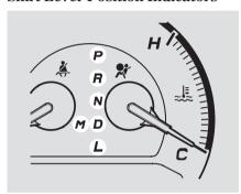
These indicators on the instrument panel show which position the shift lever is in. The illuminated number under the tachometer shows you the gear you have selected in the Sequential SportShift mode.
