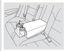
The rear beverage holder is in the rear seat armrest. Open the beverage holder by pushing the front of it, and pulling the holder all the way out.
