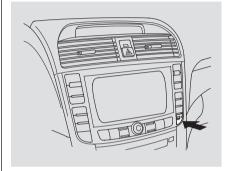
The rear window defogger clears fog, frost, and thin ice from the window. Push the defogger button to turn it on and off. The indicator in the button comes on to show the defogger is on. If you do not turn it off, the defogger will shut itself off after about 15 minutes. It also shuts off when you turn off the ignition. You have to turn it on again when you restart the vehicle.
