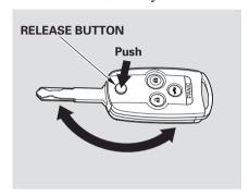
The master key can be retracted into the remote transmitter. To use the key, push the release button. The key should be fully extended. To retract the key, push the release button and at the same time push the key into the remote transmitter until it is securely latched. Always make sure the key is fully extended when you insert it to the ignition switch. If the key is not fully extended the immobilizer system may not operate properly and prevent the engine from starting.
