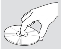
Handle a disc by its edges; never touch either surface. Do not place stabilizer rings or labels on the disc. These, along with contamination from finger prints, liquids, and feltip pens, can cause the disc to not play properly, or possibly jam in the drive.
