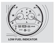
This indicator is in the fuel gauge. It comes on as a reminder that you must refuel soon. When the indicator comes on, there is about 1.2 U.S. gal  $(4.5 \ \ell)$  of fuel remaining in the tank before the needle reaches E. There is a small reserve of fuel remaining in the tank when the needle does reach E.
