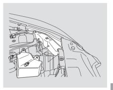
If you are replacing the bulb on the driver's side, remove the air intake cover by removing the two fastener pins and pulling the cover out. Then remove the upper part of the air intake duct by pulling it straight up.
