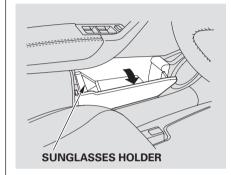
The interior of each front door has an extendable pocket for maps and other small, lightweight items. Each pocket also has a sunglasses holder. You can remove the sunglasses holder to make more room in the pocket.
