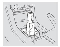
The manual transmission is synchronized in all forward gears for smooth operation. It has a lockout so you cannot accidentally shift from fifth to reverse instead of sixth (see page 251). When shifting up or down, make sure you push the clutch pedal down all the way, shift to the next gear, and let the pedal up gradually. When you are not shifting, do not rest your foot on the clutch pedal. This can cause your clutch to wear out faster.
