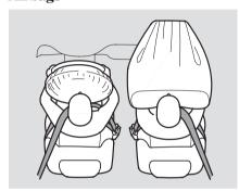
Your vehicle has a supplemental restraint system (SRS) with front airbags to help protect the heads and chests of the driver and a front seat passenger during a moderate to severe frontal collision (see page 24 for more information on how your front airbags work).
