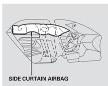
In a moderate to severe side impact, sensors will detect rapid deceleration and signal the control unit to instantly inflate the side curtain airbag on the driver's or the passenger's side of the vehicle.
