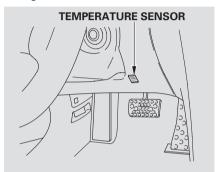
The climate control system has a temperature sensor next to the steering column. Do not cover the sensor or spill any liquid on it.
