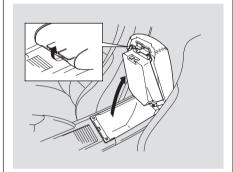
To open the console compartment storage area, pull up on the left lever, and lift the armrest. To close, lower the armrest, and push it down until it latches.
