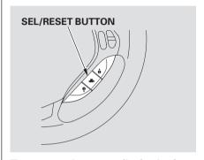
To reset a trip meter, display it, then press and hold the SEL/RESET button until the number resets to "0.0".
