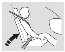
Adjust the driver's seat-back to a comfortable, upright position, leaving ample space between your chest and the airbag cover in the center of the steering wheel.
