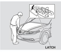
If the hood latch handle moves stiffly, or if you can open the hood without lifting the handle, the mechanism should be cleaned and lubricated.
