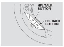
To operate the HFL, use the HFL Talk and Back buttons on the left side of the steering wheel.
