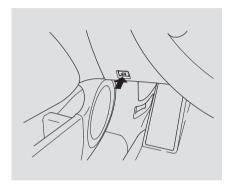
To open the trunk, press the trunk release button on the left corner of the dashboard. To open the trunk from the outside, press the trunk release button on the remote transmitter.
