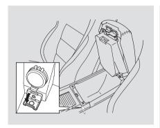
The auxiliary input jack is underneath the accessory power socket in the console compartment. The system will accept auxiliary input from standard audio accessories using a 1/8 inch stereo miniplug.
