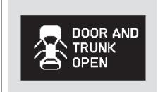
Your vehicle has a door and trunk open monitor on the multi-information display to indicate when a specific door or the trunk is not tightly closed.
