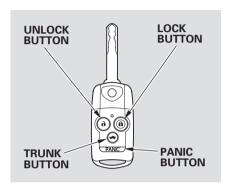
LOCK — Press this button once to lock all doors. Some exterior lights will flash. When you push LOCK twice within 5 seconds (depending on the keyless memory setting), you will hear a beep to verify that the doors are locked and the security system has set. You cannot lock the doors if any door is not fully closed or if the key is in the ignition switch.
