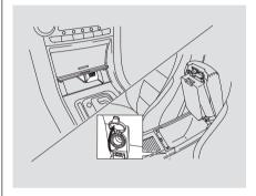
There are two accessory power sockets. One is in the front of the center console under the utility pocket lid. The other is under the armrest in the console compartment storage area.
