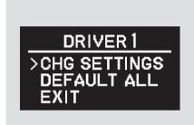
To enter the customizing mode, press the SEL/RESET button while "Keyless Memory Setting<sup>TM</sup>" is displayed. The display will change as shown above.
