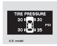
To see the inflation pressures of all four tires, press the SEL/RESET button on the steering wheel. The display changes as shown above.
