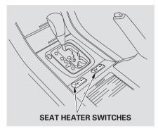
Both front seats are equipped with seat heaters. The passenger seat only has heaters in the seat bottom because of the side airbag off system. The ignition switch must be in the ON (II) position to use them. Push the HI side of the switch to rapidly heat up the seat. After the seat reaches a comfortable temperature, push the LO side of the switch. This will keep the seat warm.
