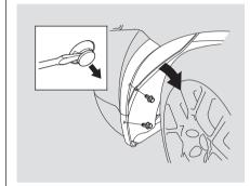
1. Start the engine. If you are replacing a driver's side bulb, turn the steering wheel all the way to the right. If you are replacing a passenger's side bulb, turn the steering wheel to the left. Turn off the engine.
