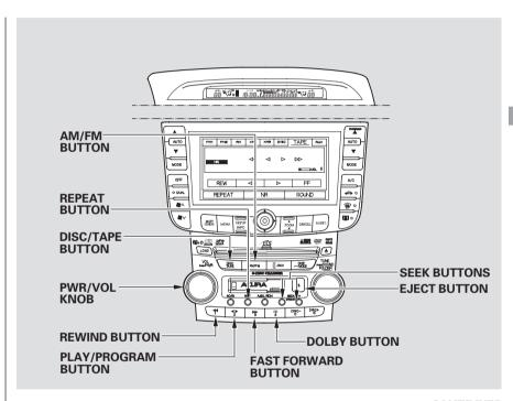
Dolby\* noise reduction turns on when you insert a tape. The "NR" indicator will come on in the display. If the tape was not recorded in Dolby, turn it off by pressing the
