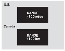
When you press the INFO (▼) button, the display changes as shown above. This is the estimated distance you can travel on the fuel remaining in the tank. This distance is estimated from the fuel economy you received over the last several miles (kilometers), so it will vary with changes in speed, traffic, etc. It measures miles in U.S. models and kilometers in Canadian models.
