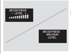
To reduce glare at night, the instrument panel illumination dims when you turn the light switch to ₹00 or ≣□ . Pressing the MAX button will bring it to the maximum level.
