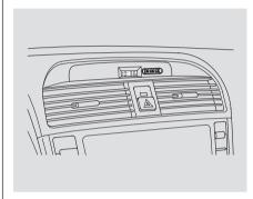
On models without navigation system The clock displays the time with the ignition switch in the ON (II) position. If your vehicle's battery is disconnected or goes dead, you will need to reset the clock.
