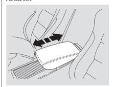
The lid of the console compartment can be used as an armrest by moving it forward and backward. Make sure the armrest is securely latched.
