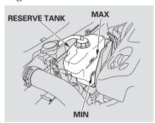
Look at the coolant level in the radiator reserve tank. Make sure it is between the MAX and MIN lines. If it is below the MIN line, see **Adding Engine Coolant** on page 286 for information on adding the proper coolant.
