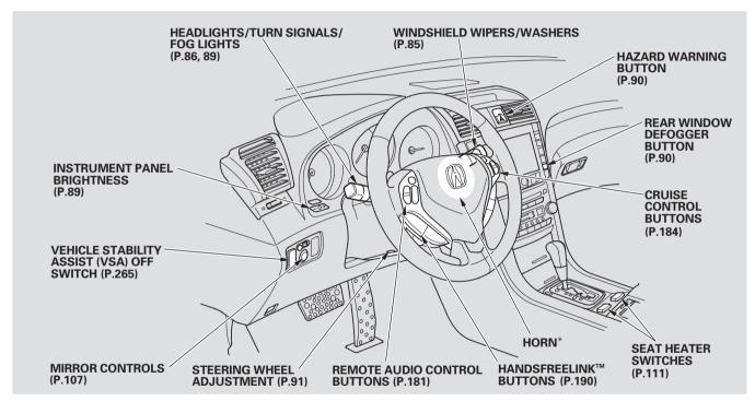
\* : To use the horn, press the center pad of the steering wheel.
