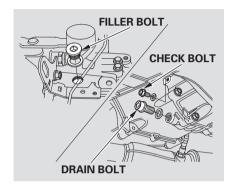
Check the fluid level with the transmission at normal operating temperature and the vehicle sitting on level ground. Remove the check bolt, and look for transmission fluid coming out of the bolt hole. If a small amount of fluid drips out of the bolt hole, reinstall the check bolt.
