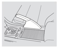
To apply the parking brake, pull the lever up fully. To release it, pull up slightly, push the button, and lower the lever. The parking brake indicator on the instrument panel should go out when the parking brake is fully released (see page 59).
