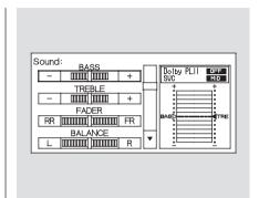
**Fader** — Adjusts the front-to-back strength of the sound. To adjust the front/rear fader, touch the FR or RR icon.
