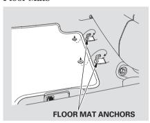
The driver's and right rear passenger's floor mats that came with your vehicle hook over the floor mat anchors. This keeps the floor mats from sliding forward and possibly interfering with the pedals (driver's floor mat) or with the seat weight sensors (right rear floor mat).
