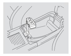
The coin holder inside the console compartment is removable. To remove it, pull it up. The coin holder can also be stored in either front door pocket.
