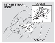
1. After properly securing the child seat (see page 45), lift the head restraint, then route the tether strap over the seat-back and through the legs of the head restraint.
