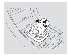
In Sequential SportShift mode, each time you push forward on the shift lever, the transmission shifts to a higher gear. Pull back on the lever to downshift. The number of the gear selected is displayed on the instrument panel.
