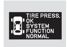
When the tire pressure monitoring system (TPMS) is functioning normally and the tires are properly inflated, you will see the above display on the multi-information display as it cycles through its main menu.
