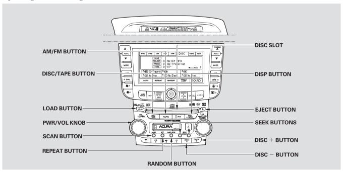
Your vehicle's audio system has an in-dash disc changer that holds up to six discs. You operate this disc changer with the same controls used for the radio. To operate the disc changer, the ignition switch must be in the ACCESSORY (I) or ON (II) position.
