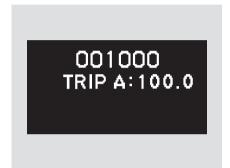
The odometer shows the total distance your vehicle has been driven. It measures miles in U.S. models and kilometers in Canadian models. It is illegal under U.S. federal law and Canadian provincial regulations to disconnect, reset, or alter the odometer with the intent to change the number of miles or kilometers indicated.
