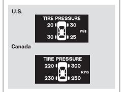
To see the inflation pressures of all four tires, press the SEL/RESET button. The display changes as shown above.
