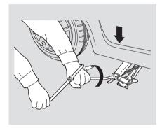
12.Lower the vehicle to the ground, and remove the jack.
