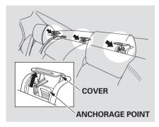
A child seat with a tether can be installed in any seating position in the back seat, using one of the anchorage points shown above.
