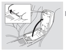
You can put small items in the tray located in the console compartment lid. To use the tray, pull up on the right lever and lift up the armrest.
