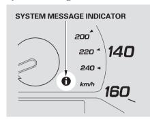
If there is a problem with your vehicle, for example, the parking brake is not fully released or a door is not fully closed, the multi-information display will show you the problem. It does this by interrupting the current display with one or more messages.
