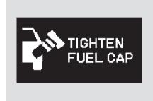
Your vehicle's on board diagnostic system will detect a loose or missing fuel fill cap as an evaporative system leak. The first time a leak is detected a "TIGHTEN FUEL CAP" message appears on the multi-information display. Turn the engine off, and confirm the fuel fill cap is installed. If it is, loosen it, then retighten it until it clicks at least once. The message should go off after several days of normal driving once you tighten or
