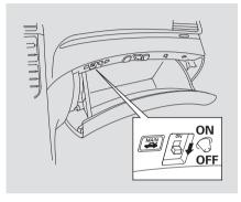
To protect items in the trunk, you can disable the trunk-release button on the dashboard by turning off the trunk main switch in the glove box, locking the glove box, and locking the trunk pass-through cover with the master key.
