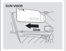
To use the sun visor, pull it down. When using the sun visor for the side window, remove the support rod from the clip, and swing it out. In this position, the sun visor can be adjusted by moving it on its slider.
