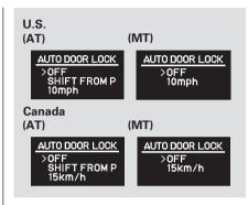
Select the desired condition by moving the pointer with the INFO (▼) button and enter your selection by pressing the SEL/RESET button.
