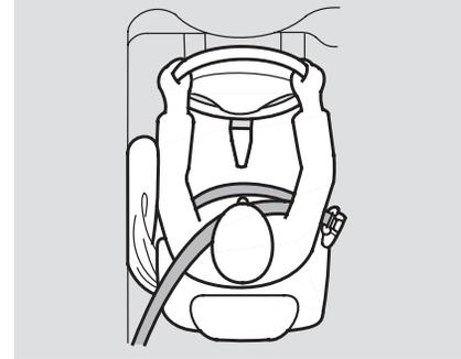
If you ever have a moderate to severe side impact, sensors will detect rapid acceleration and signal the control unit to instantly inflate either the driver's or the passenger's side airbag and activate the seat belt tensioner on that side of the vehicle.
