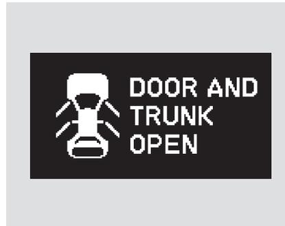
Your vehicle has a door and trunk open monitor on the multi-information display to indicate when a specific door or the trunk is not tightly closed.
