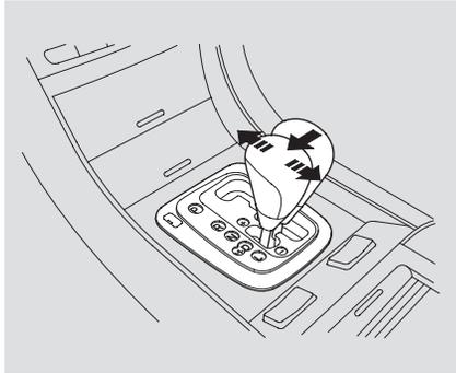
In Sequential SportShift mode, each time you push forward on the shift lever, the transmission shifts to a higher gear. Pull back on the lever to downshift. The number of the gear selected is displayed on the instrument panel.
