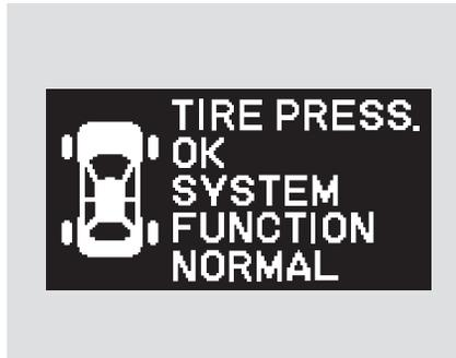
When the tire pressure monitoring system (TPMS) is functioning normally and the tires are properly inflated, you will see the above display on the multi-information display as it cycles through its main menu.
