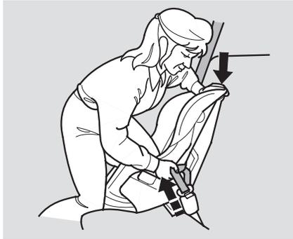
4. After confirming that the belt is locked, grab the shoulder part of the belt near the buckle, and pull up to remove any slack from the lap part of the belt. Remember, if the lap part of the belt is not tight, the child seat will not be secure.
