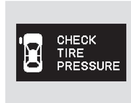
Each tire has its own pressure sensor. If the air pressure of a tire becomes significantly low, the sensor in that tire immediately sends a signal that causes the low tire pressure indicator in the instrument panel to come on. If this happens, you will see which tire is losing pressure on the multi-information display along with a "CHECK TIRE PRESSURE" message.
