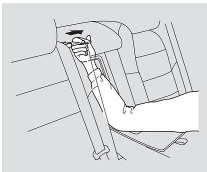
If your vehicle's battery goes dead or is disconnected, you can open the trunk from the rear seat by pulling the trunk release handle. Reach the handle through the trunk pass-through.
