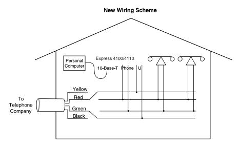
Figure 2-1. Wiring Scheme 1: Use existing analog telephone equipment, but replace single analog telephone service with ISDN service
