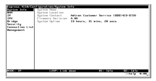
Figure 3-2. Configuration/System Info Screen
