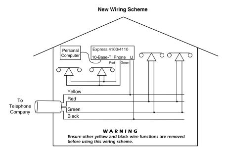
Figure 2-2. Wiring Scheme 2: Retain single analog telephone service and add ISDN service
