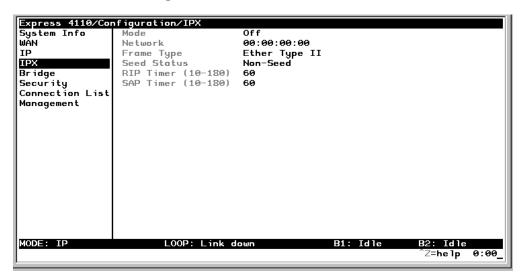
Figure 3-5. Configuration/IPX Screen
