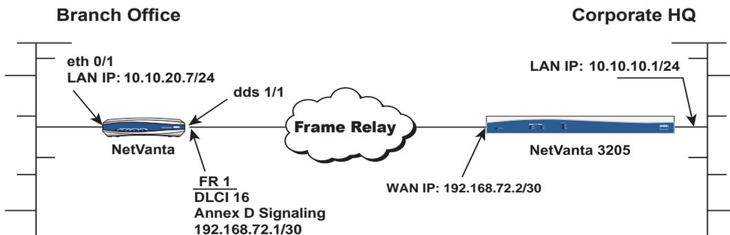
PPP over DDS Connection Diagram
