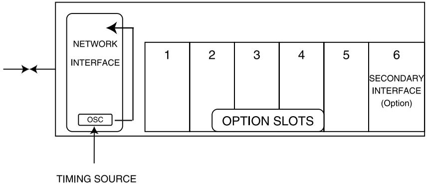
**Figure 4-8. Internal Clock Source**
