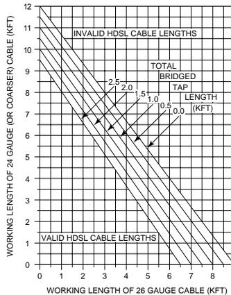
**Figure F-1. HDSL Deployment Guidelines**
