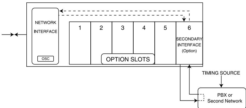
**Figure 4-9. Secondary Clock Source**
