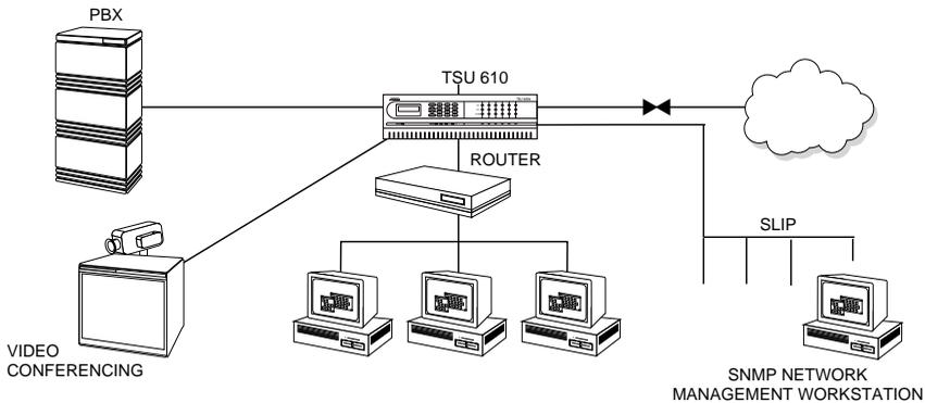
**Figure 1-2. Router, PBX, Video Conferencing Application Set Up**
