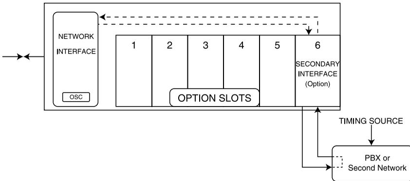
**Figure 5-9. Secondary Clock Source**
