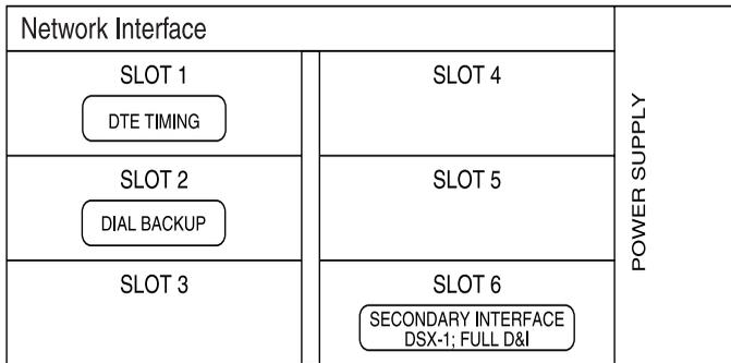
**Figure 2-6. TSU 610 Slot Designation (Rear View)**
