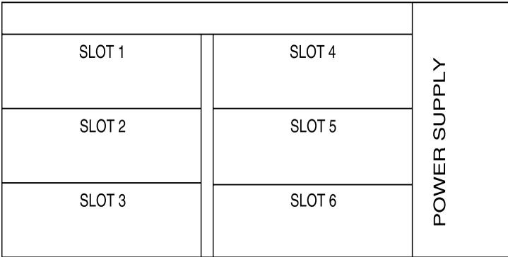
**Figure 3-2. Module Slots, TSU 610**
