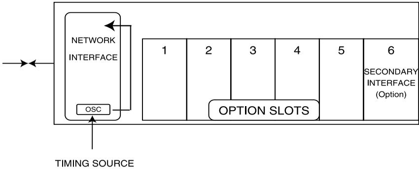
**Figure 5-8. Internal Clock Source**
