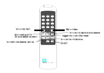
The Voice  $^{TM}$  Plus can be operated by the included infrared remote control, so you don't have not to be close to the base unit when performing such common operations as dialing or answering a phone call.
