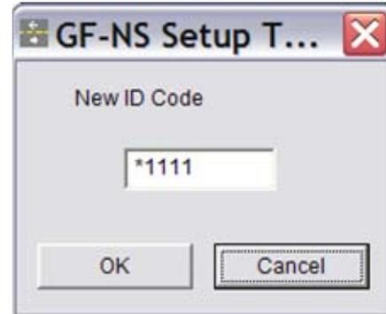
This is a security code and is required in order to make any changes to the GF-NS/A data via the keypad, or when exporting data into the unit.
