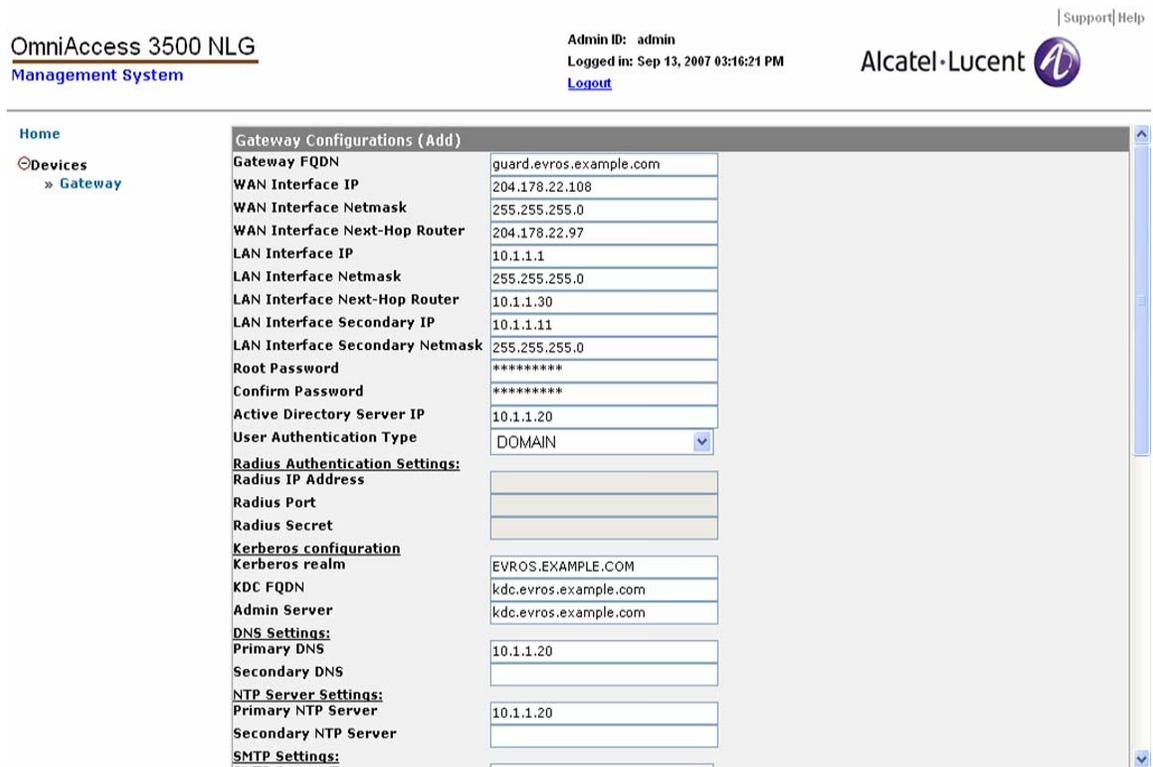
Figure 10 - Gateway Configuration (Add)
