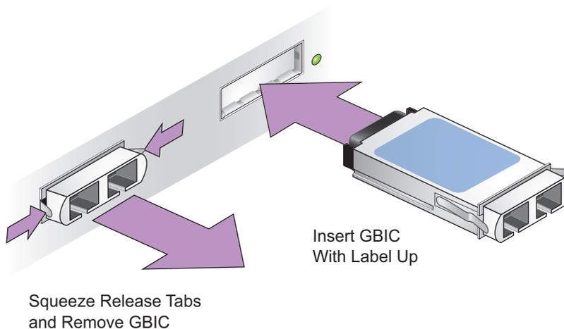
**FIGURE 3-1** GBIC Removal and Insertion
