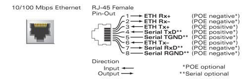
The port accepts a 4- or 8-conductor Category 5 UTP Ethernet cable with an RJ-45 male connector. A straight-through cable is required for connection to a network port. A crossover cable is required for connection to a management workstation.
