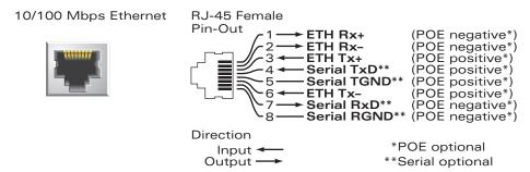
The port accepts a 4- or 8-conductor Category 5 UTP Ethernet cable with an RJ-45 male connector. A straight-through cable is required for connection to a network port. A crossover cable is required for connection to a management workstation.
