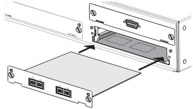
**Caution:** The slide-in modules are **not** hot-swappable. Be sure you power off the switch before installing any of these modules.
