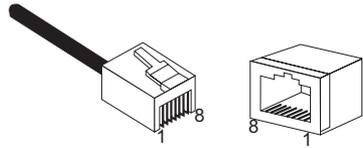
For 100BASE-TX/10BASE-T connections, a twisted-pair cable must have two pairs of wires. Each wire pair is identified by two different colors. For example, one wire might be red and the other, red with white stripes. Also, an RJ-45 connector must be attached to both ends of the cable.
