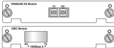
**Warning:** This switch uses lasers to transmit signals over fiber optic cable. The lasers are compliant with the requirements of a Class 1 Laser Product and are inherently eye safe in normal operation. However, you should never look directly at a transmit port when it is powered on.
