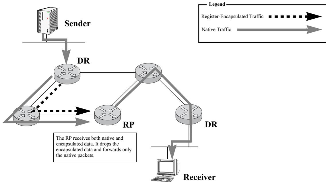
A register-stop packet is sent back to the sender's DR to prevent the DR from unnecessarily encapsulating the packets. Once the register-encapsulated packets are discontinued, the packets flow natively from the sender to the RP—along the source-specific tree to the RP and, from there, along the shared tree to all receivers.
