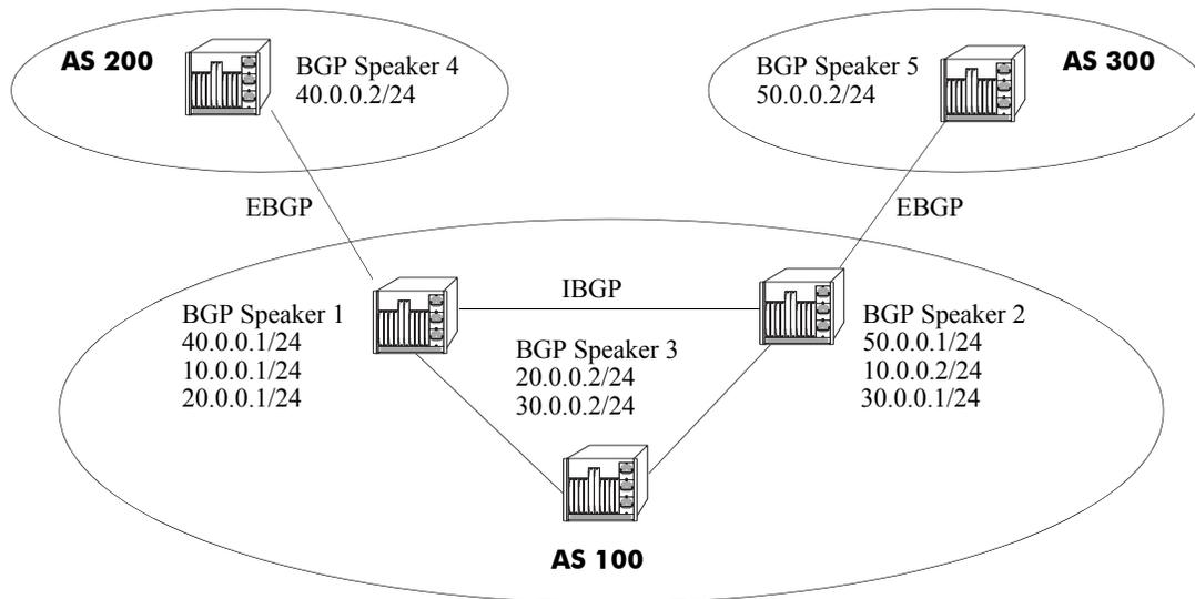
In the above network, Speakers 1, 2, and 3 are part of AS 100 and are fully meshed. Speaker 4 is in AS 200 and Speaker 5 is in AS 300.
