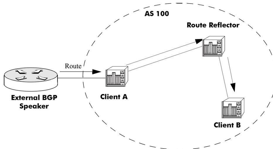
The internal peers of a route reflector are divided into two groups: client peers and non-client peers. The route reflector sits between these two groups and reflects routes between them. The route reflector, its *clients*, and *non-clients* are all in the same autonomous system.
