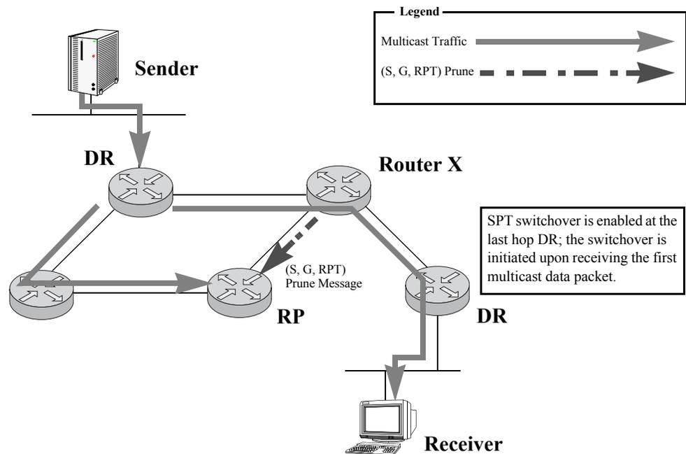
The Receiver is now receiving multicast traffic along the Shortest Path Tree between the Receiver and the Source.
