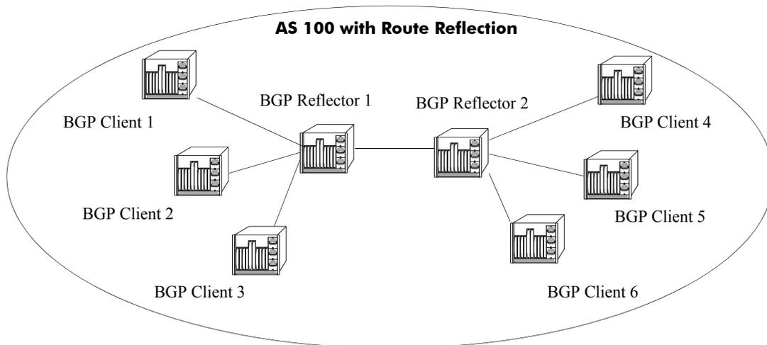
In the diagram above, Clients 1, 2, and 3 peer with Reflector 1, and Clients 4, 5, and 6 peer with Reflector 2. Reflector 1 and 2 peer with each other. This allows each BGP speaker to maintain only one BGP session, rather than a possible seven sessions, as demonstrated below:
