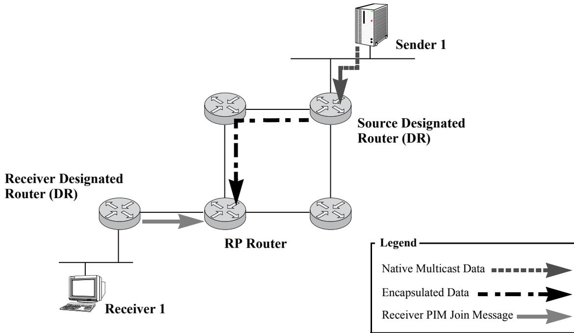
Once the distribution tree for group G is learned at the RP, the encapsulated data being sent from the source DR are now unencapsulated at the RP and forwarded natively to the Receiver.
