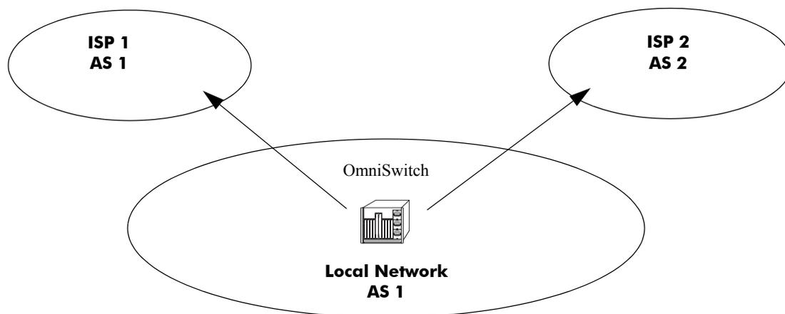
BGP is intended for use in networks with multiple autonomous systems. It is not intended to be used as a LAN routing protocol, such as RIP or Open Shortest Path First (OSPF). In addition, when BGP is used as an internal routing protocol, it is best used in autonomous systems with multiple exit points as it includes features that help routers decide among multiple exit paths.
