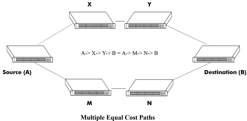
Delivery of packets along equal paths is based on flows rather than a round-robin scheme. Equal cost is determined based on standard routing metrics. However, other variables, such as line speed, are not considered. So it is possible for OSPF to decide two paths have an equal cost even though one may contain faster links than another.
