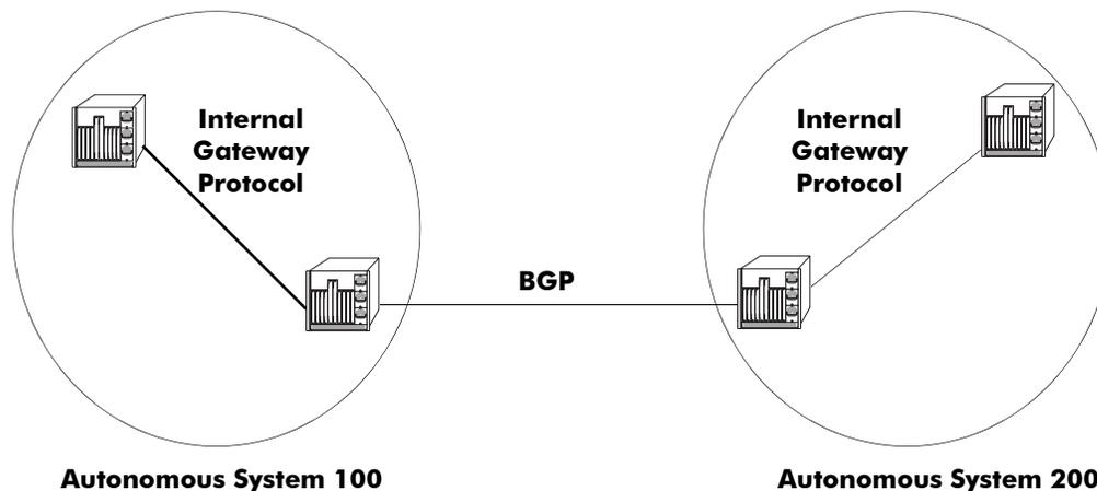
Each AS has a number assigned to it by an Internet Registry, much like an IP address. BGP is the standard Exterior Gateway Protocol (EGP) used for exchanging information between ASs.
