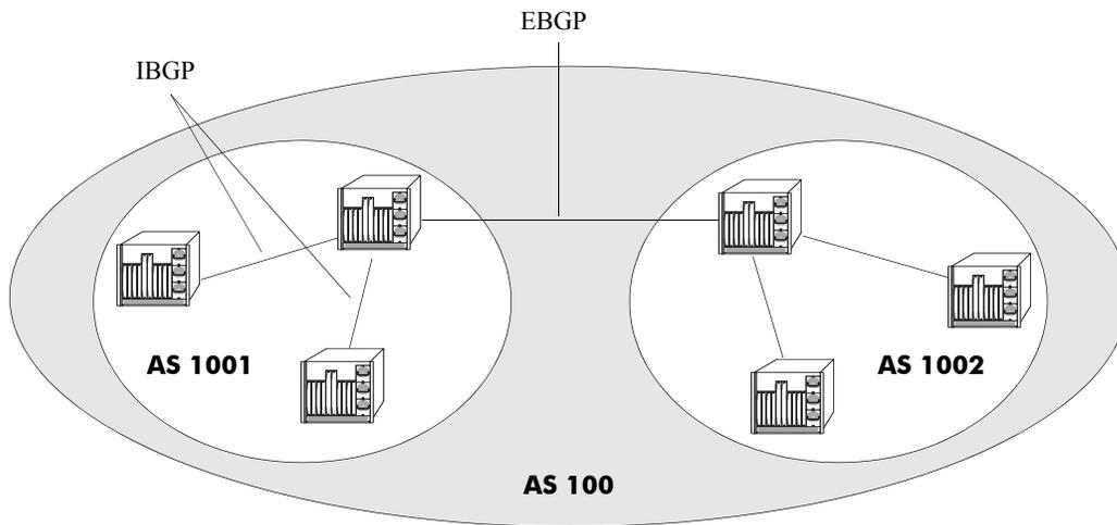
AS 100 is now a confederation consisting of AS 1001 and AS 1002. Even though EBGP is used to communicate between AS 1001 and 1002, the entire confederation behaves as though it were using IBGP. In other words, the sub AS attributes are preserved when crossing the sub AS boundaries.
