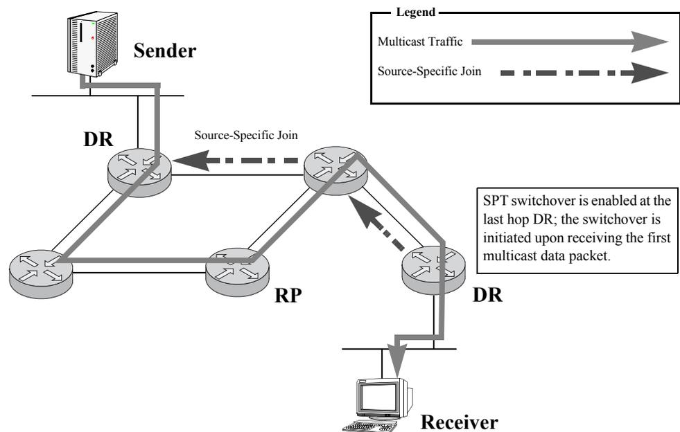
Once the Sender's DR receives the (S,G) Join message, the DR sends the multicast packets natively along the Shortest Path Tree. At this point, Router X (the router shown between the Sender's DR and the Receiver's DR) will be receiving two copies of the multicast data—one from the SPT and one from the RPT. This router drops the packets arriving via the RP tree and forwards only those packets arriving via the SPT.
