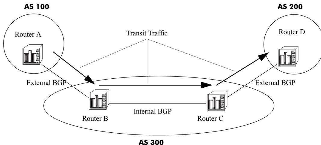
In the above diagram, AS 100 and AS 200 can send and receive traffic via AS 300. AS 300 has become a transit AS using IBGP between Router B and Router C.
