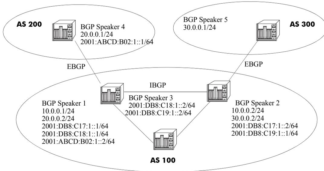
In the above network, Speakers 1, 2, and 3 are part of AS 100 and are fully meshed. Speaker 4 is in AS 200. Speaker 3 is part of a homogenous IPv6 network domain (i.e. pure IPv6 network), internal to AS 100. Speaker 5 in AS 300 is not aware of IPv6 capabilities.
