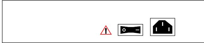
**BPS-DC-PS-250** A 48 volt (input voltage) DC version of the BPS-AC-PS-250 power supply. This power supply has a capacity of 50 Amps and can provide 250 Watts of power at 5 Volts. It requires the use of 12 to 14 gauge wire for connections to the DC power source. It supports an input voltage range of -40 to -60 VDC (-48 VDC nominal). It can support any possible combination of switches.
