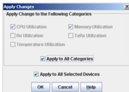
Notice that the Apply Changes Window for multiple devices is slightly different than the Apply Changes Window for a single device. In the Apply Changes Window for multiple devices, each of the monitored items is grayed out, and **Apply to All Categories** and **Apply to All Selected Devices** options are enabled.
