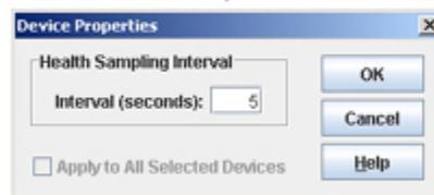
**Note:** If you select more than one switch, the "Apply to All Selected Devices" box will be checked. Edit the "Interval" field and click **OK**. The sampling interval will be updated for all of the selected switches.
