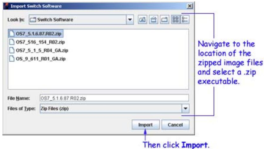
Messages in the Status Panel report the start, progress, and finish of the import process, and report any error that may occur. When the process is complete, the imported firmware files are listed in the Upgrade Image tab.
