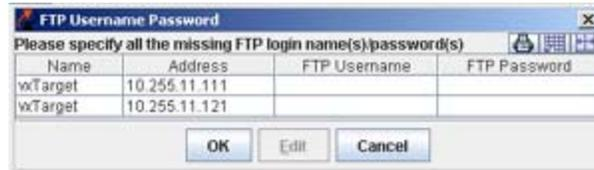
6. Select a device in the **FTP Username Password** window and click the **Edit** button. The Specify FTP Logic window displays, shown below. Enter the FTP user name and password for the selected device in the appropriate fields. If the user name and password you enter also apply to the other devices, click the **Same for all Unspecified** checkbox. Then click the **OK** button.
