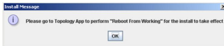
AOS switches can be rebooted from OmniVista's Topology application, by connecting to the switch and using the **Load From** command. Refer to the Topology help for more information. XOS switches can be rebooted via Telnet, etc. The OmniStack 6024, 6048, 6124, 6148, and 8008 will automatically reboot without user intervention when the file transfer is complete.
