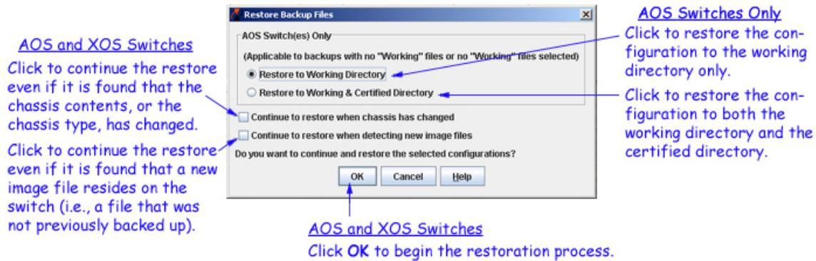
5. For both AOS and XOS switches, click the **OK** button to start the restoration process. When the restore is complete, a message reports the success or failure of the operation in the status panel.
