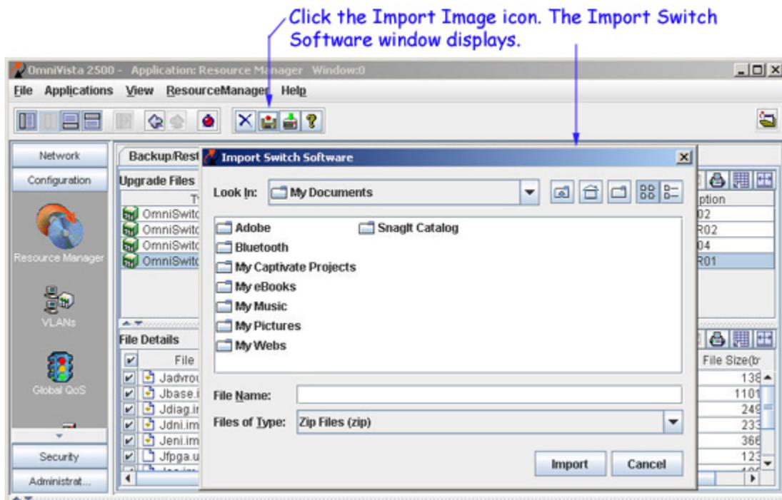
3. In the Import Switch Software window, navigate to the location of the zipped firmware files and select a .zip executable. Then click the **Import** button. The import process begins immediately.
