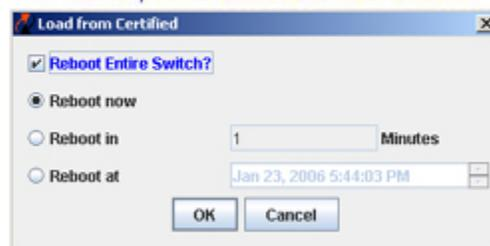
**Note:** When you select the **Reboot Entire Switch** option the operation does not necessarily take place immediately since OmniVista needs to propagate the command to all switches you have upgraded.
