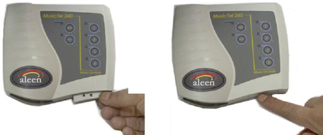
**Figure 2-3. Inserting Memory Module**
