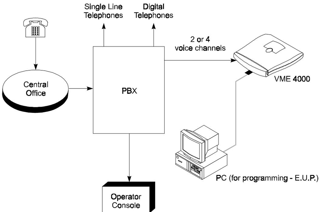
**Figure 2-6 System Installation**
