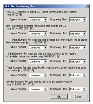
Figure 25. PRI ISDN Numbering Plan dialog box
