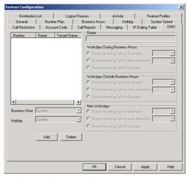
Figure 19. DNIS window, System Configuration
