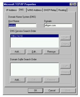
Figure 3. DNS Configuration window
