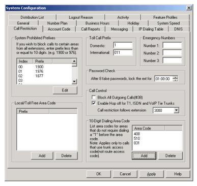
Figure 11. Call Restriction window, System Configuration
