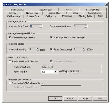
Figure 16. Messaging window, System Configuration
