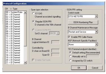
Figure 21. PRI Protocol Configuration window
