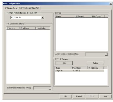
Figure 4. VoIP Codec Configuration window
