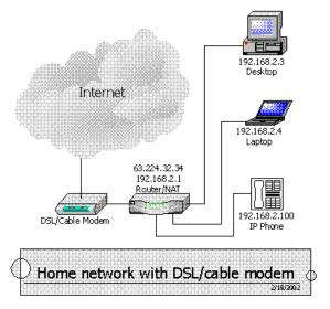
Figure 7. Home Network with DSL/Cable Modem
