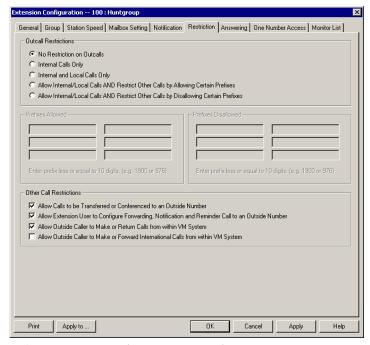
Figure 15. Restriction window, Extension Configuration
