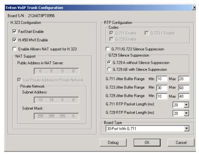
Figure 12. Triton VoIP Trunk Configuration window
