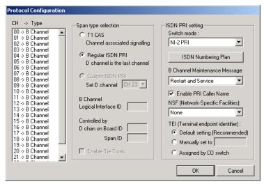
Figure 20. T1/PRI Protocol Configuration window
