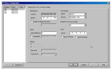
Figure 1. IP Phone Configuration window, General tab
