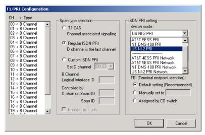
Figure 23. ISDN PRI Switch Mode
