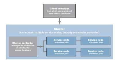
Example of a network setup for distributed rendering
