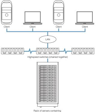
cluster controller and render-only Shake service nodes, plus rackmounted shared storage device.
