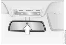
rear of the mirror. Refrain from attaching stickers or other objects to the windshield in the area immediately behind the rearview mirror.
