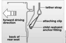
Depending on the location selected for seating in the rear passenger area, attach the tether strap to the corresponding anchorage point to secure the child-restraint system, as shown in the illustration.
