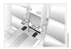
When reattaching the cover, guide both bars into the guide and press the cover back into place. Secure the safety belts in their holders again. ◀
