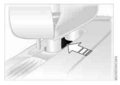
Using a screwdriver from the onboard tool kit, remove the cover panel; to do this, position the screwdriver under the notch
