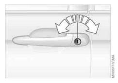
Whenever closing the windows or sliding/tilt sunroof you should always monitor their path and progress to ensure that no one is injured. Releasing the key stops the operation.
