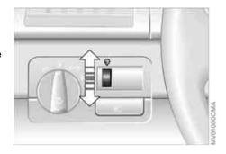
Turn the rotary dial with the parking/ low beam lamps on to adjust the illumination intensity.
