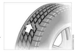
wall with TWI – Tread Wear Indicator. At a tread depth of 1/16 in / 1.6 mm, the indicators signal that the legally permissible wear limit has been reached.
