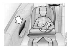
This is the right way a child should sit in a child restraint when rear side airbags are provided.
