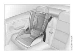
The belt cannot be extracted further. Always observe the installation instructions provided by the manufacturer of the child-restraint system.
