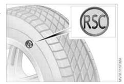
Run Flat tires are labeled on the sidewall with a circular symbol containing the letters RSC. Run Flat tires consist of self-supporting tires and special rims. The tire reinforcement ensures that driving remains possible to a restricted degree in the event of pressure drop or even if the tire is deflated.
