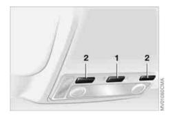
The interior lamps operate automatically.
