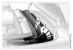
4. Grasp the convertible top by the lateral guide section – see arrow 1 – and the front convertible top frame – see arrow 2. Lift out the top and swing it forward until you encounter a perceptible resistance – until it stops. Position the rear convertible top frame vertically and close the convertible top compartment lid. Fold down the rear convertible top frame
