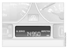
A flashing message and a "-" in front of the number mean that the service interval has already been exceeded by the distance shown on the display. Please contact your BMW center for an appointment.
