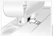
2. Push the lever toward the front of the vehicle and keep it in this position
