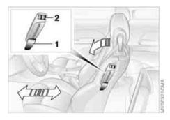
The seat-integrated safety belt system allows for easy access to the rear.
