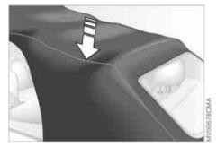
4. Position the rear convertible top frame vertically and grip it firmly
