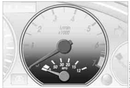
Indicates the current fuel consumption in mpg – in liters/100 km on Canadian models. This allows you to see whether your current driving style is conducive to fuel economy with minimum exhaust emissions.
