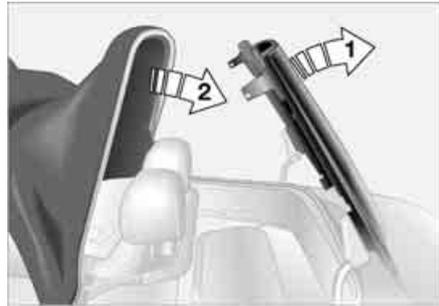
5. Reach into the recess created when the convertible top compartment lid is lifted and pull it all the way up by hand – see arrow 1
