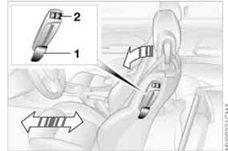
The seat-integrated safety belt system allows for easy access to the rear.
