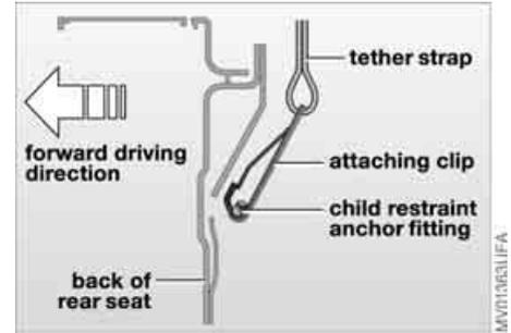
Depending on the location selected for seating in the rear passenger area, attach the tether strap to the corresponding anchorage point to secure the child-restraint system, as shown in the illustration.
