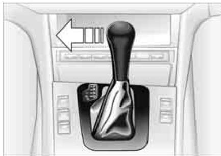
The transmission will only execute upshifts and downshifts that will result in an appropriate combination of vehicle speed and engine rpm. For instance, downshifts that would result in excessive engine speed are not executed. The desired, then the actual gear, briefly appear in the instrument cluster.
