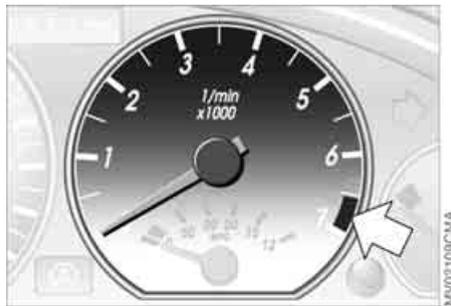
Do not operate the engine with the needle in the red overspeed zone of the gauge.
