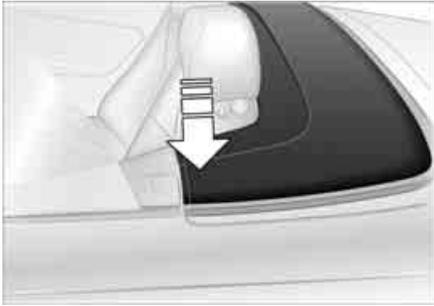
As soon as the convertible top compartment lid closes the central locking system will release the lock to allow renewed access to the luggage compartment.
