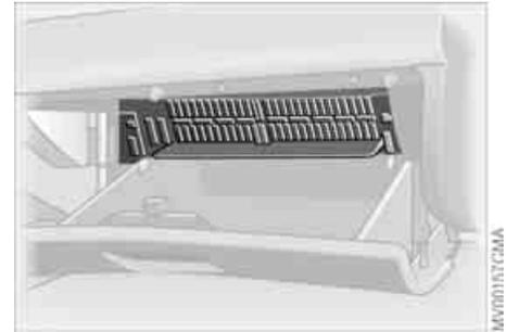
You will find the fuses and information on their respective allocation in the glove compartment behind a panel with two snap clips.
