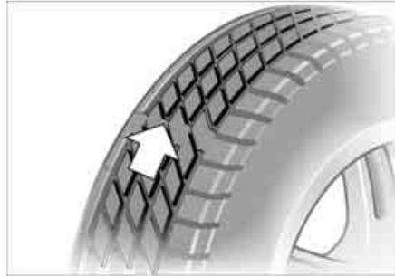
wall with TWI – Tread Wear Indicator. At a tread depth of 1/16 in / 1.6 mm, the indicators signal that the legally permissible wear limit has been reached.
