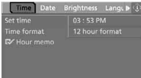
5. Select "Set time" and press the controller. The hours are highlighted.
