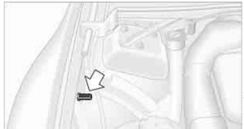
5. Attach the second terminal clamp of the minus- jumper cable to the negative terminal of the battery or to an engine or body ground of the assisting vehicle.
