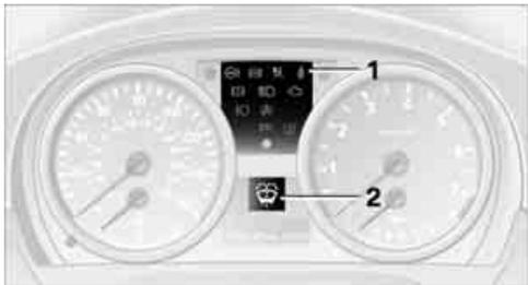
Indicator and warning lamps can light up in various combinations and colors in both the indicator area **1** and the display **2**.
