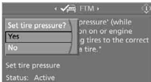
8. Start to drive. "Status: Active" reappears in the Control Display. Initialization is then completed while the car is in motion.
