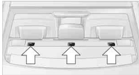
If you use a child-restraint system with a tether strap, three additional tether anchorage points have been provided, refer to the arrows in the illustration. Depending on the location selected for seating in the rear passenger area, attach the tether strap to the corresponding anchorage point to secure the child-restraint system, as shown in the illustration below.
