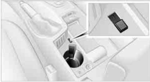
The storage compartment in the center armrest can be ventilated: push the switch to position 1.
