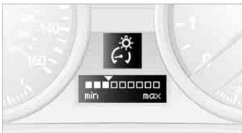
3. Lightly push button 1 up or down to select the brightness; the setting is stored immediately.
