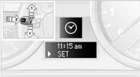
1. Lightly push button **1** in the turn indicator stalk repeatedly up or down until the appropriate symbol appears in the display, accompanied by the time and the word "SET".
