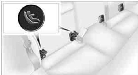
The anchorage points for the LATCH child-restraint fixing system are located behind the indicated protective caps. Flip up the corresponding caps.
