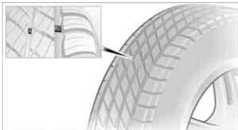
Wear indicators in the base of the tread groove are distributed around the tire's circumference; the letters TWI, Tread Wear Indicator, on the tire's sidewalls identify tires that incorporate these wear indicators. Once the tire tread has worn down to the wear indicators, the tire has worn to a depth of 1/16 in/1.6 mm.
