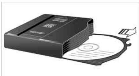
When loading CDs into or removing them from the CD magazine, hold them at the edge and do not touch the reflective signal-sensing area.
