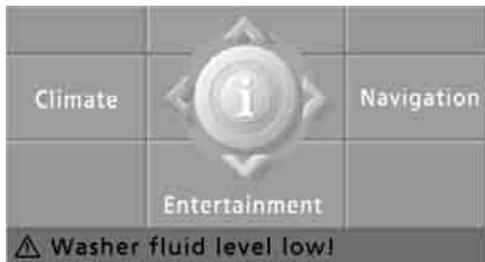
Text messages at the lower edge of the Control Display explain the meaning of the displayed indicator and warning lamps.
