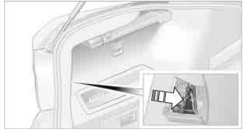
1. Using a screwdriver, pry off the cover in the luggage compartment or release the turnlock fastener by turning it counterclockwise and remove the cover.
