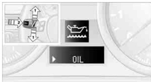
1. Lightly push button **1** in the turn indicator stalk repeatedly up or down until the appropriate symbol is shown in the display, accompanied by the word "OIL".
