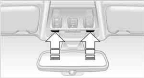
There are reading lamps at the front and rear\*, next to the interior lamps. To switch on and off, press the button briefly.
