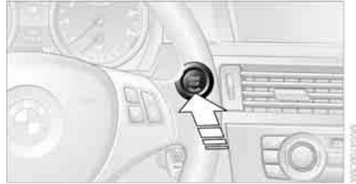
Each time the start/stop button is pressed, radio readiness or the ignition is switched on or off.
