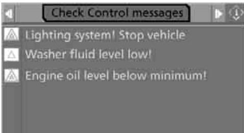
Some Check Control messages remain visible until the malfunction in question has been rectified. They cannot be hidden. If several malfunctions occur at the same time, the Check Control messages are displayed in succession.
