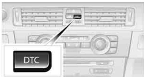
Press the button and hold it down for at least 3 seconds; the DSC indicator lamps in the
