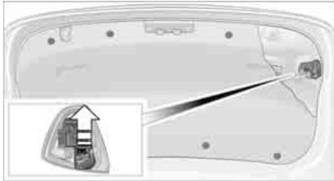
1. Pry out the plastic plugs in the trim of the luggage compartment lid using a screwdriver and remove the trim.
