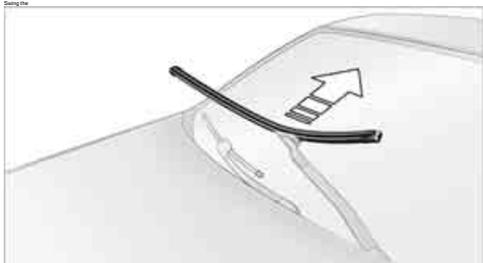
3. Fold the wiper blade upwards.
