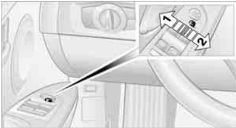
1. Push the mirror selector switch to the position for the driver's-side mirror 1.
