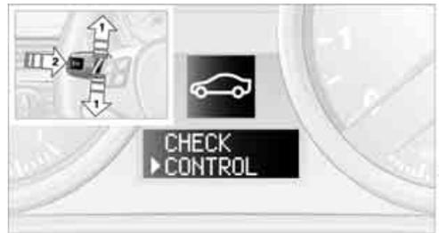
1. Lightly push button 1 in the turn indicator stalk repeatedly up or down until the appropriate symbol appears in the display, accompanied by the words "CHECK CONTROL".
