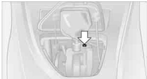
3. Using the screwdriver from the onboard tool kit, refer to page 187, hold down the red lever and move the selector lever to the desired position in the usual way.
