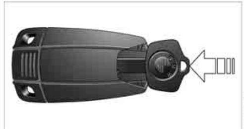
The adapter is necessary for starting the car with the spare key or switching on radio readiness.
