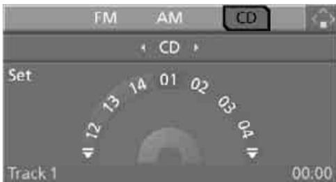
4. On cars with a CD changer, select "CD" and press the controller to start the CD player.
