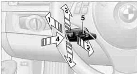
Press the lever upward or downward, arrow **3**. The displays in the speedometer disappear.
