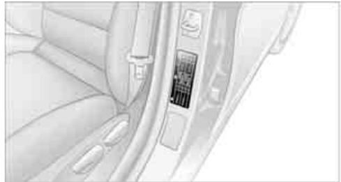
The inflation pressures for your factory-installed tires at ambient temperature can be found on the door post when you open the driver's door.
