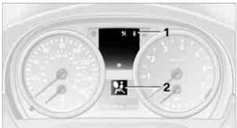
Indicator and warning lamps can light up in both the indicator area **1** and the display **2** in various combinations and colors.
