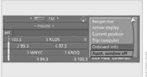
To turn back on, switch to the assistance window and press the controller.
