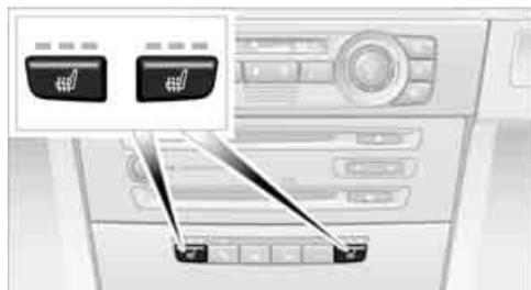
Press once for each temperature level. Three lamps indicate the highest temperature.
