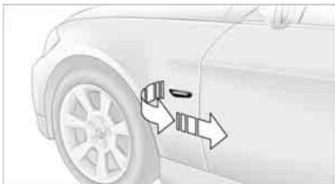
1. Press back against the front edge of the light with the tip of your finger, then pivot it out.
