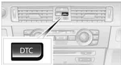
Briefly press the button; the DTC indicator lamps in the instrument cluster come on.
