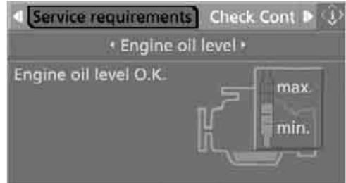
5. Select "Engine oil level" and press the controller. The oil level is displayed.
