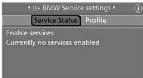
6. Select "Enable services" and press the controller. TeleService and, if applicable, BMW Assist are enabled; data exchange with the service center starts.
