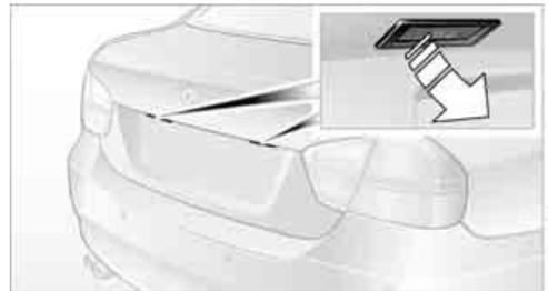
1. Using a screwdriver, push the lamp to the left in the flap of the lamp housing.
