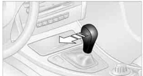
Move selector lever from position D toward the left into the M/S shifting slot:
