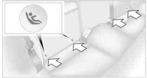
The anchorage points for the LATCH child-restraint fixing system are located underneath the identifying symbols.
