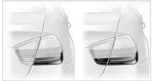
The brake lamps light up in two stages, depending on how sharply you apply the brakes.
