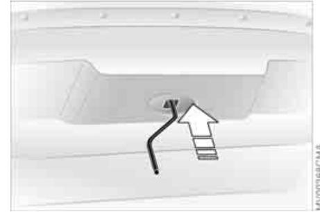
5. Use a screwdriver to lift out the cover panel that is in the center of the front convertible top frame
