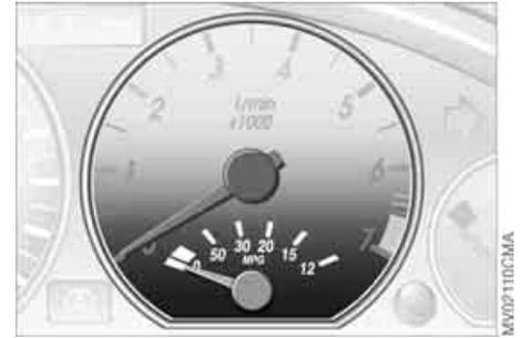
Indicates the current fuel consumption in mpg – in liters/100 km on Canadian models. This allows you to see whether your current driving style is conducive to fuel economy with minimum exhaust emissions.
