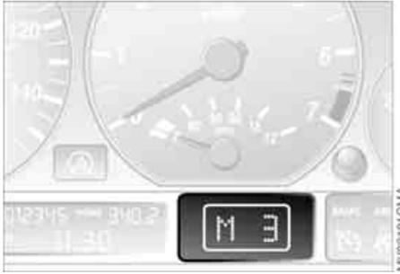
If the indicator lamp does not go out, you can place the selector lever in all positions. However, the vehicle will now only operate in 3rd and 4th gear.
