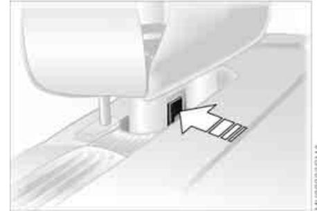
1. Using a screwdriver from the onboard tool kit, remove the cover panel; to do this, position the screwdriver under the notch
