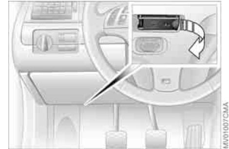
The interface socket for onboard diagnostics is located on the left-hand side of the driver's side, behind a specially marked cover located beneath the instrument panel. The cover has the letters OBD on it.
