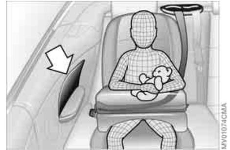
This is the right way a child should sit in a child restraint when rear side airbags are provided.
