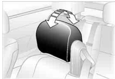
Tilt angle: position the head restraints manually in the preferred position.
