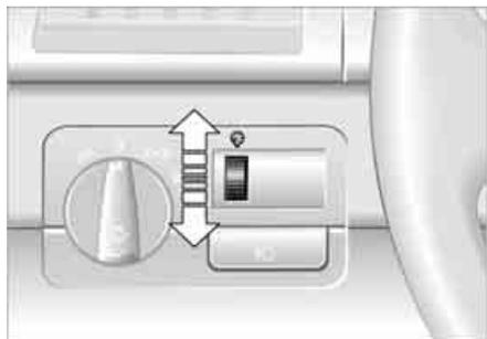
Turn the rotary dial with the parking/low beam lamps on to adjust the illumination intensity.
