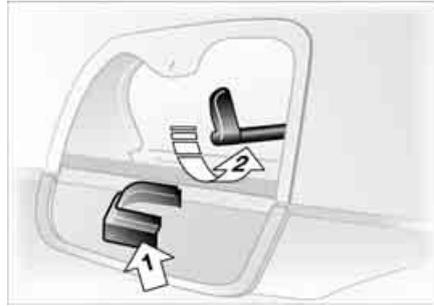
5. Before installing, first flip the cover panels that are located underneath the left and right interior lamps down. To do this, press on the slight bump on the cover panel. There is a holder in the cover panel to securely store the trim pieces that have been removed – see arrow 1
