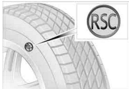
Run Flat tires are labeled on the sidewall with a circular symbol containing the letters RSC. Run Flat tires consist of self-supporting tires and special rims. The tire reinforcement ensures that driving remains possible to a restricted degree in the event of pressure drop or even if the tire is deflated.
