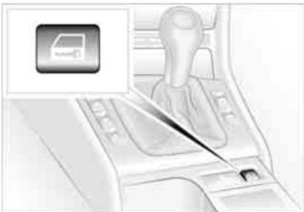
You can use this button to control the central locking system whenever the doors are closed. The doors and luggage compartment lid are unlocked or locked only. The anti-theft system is not activated.
