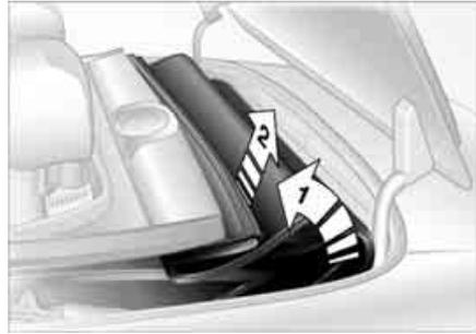
4. Grasp the convertible top by the lateral guide section – see arrow 1 – and the front convertible top frame – see arrow 2. Lift out the top and swing it forward until you encounter a perceptible resistance – until it stops. Position the rear convertible top frame vertically and close the convertible top compartment lid. Fold down the rear convertible top frame
