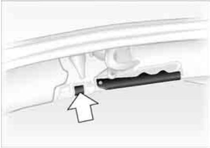
4. Open the two locking levers at the front. Press on the buttons to do so. The levers will release slightly. Open the levers as far as possible
