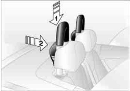
3. Keep pressing down on the protective bar – see arrow 1 – from on top until you hear it click into place
