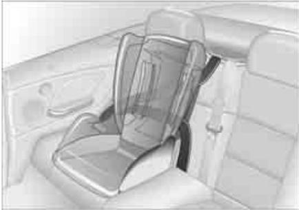
The belt cannot be extracted further. Always observe the installation instructions provided by the manufacturer of the child-restraint system.
