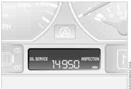
A flashing message and a "-" in front of the number mean that the service interval has already been exceeded by the distance shown on the display. Please contact your BMW center for an appointment.
