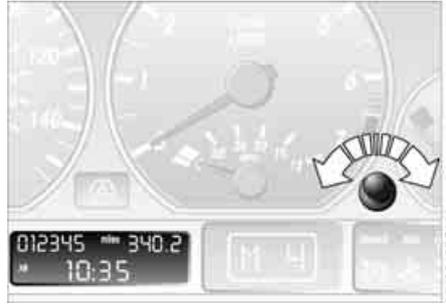
Every time you press the button, the clock display alternates between the 12-hour and 24-hour mode.
