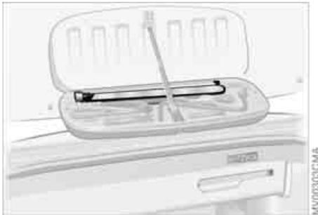
The hazard warning triangle is stored in the luggage compartment lid inside the container for the onboard tools.
