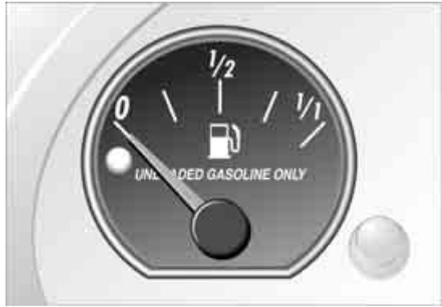
Once the indicator lamp stays on continuously, there are still approx. 2.1 gallons/8 liters of fuel in the fuel tank.
