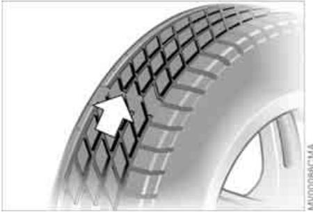
TWI, Tread Wear Indicator. At a tread depth of 1/16 in/1.6 mm, the indicators signal that the legally permissible wear limit has been reached.
