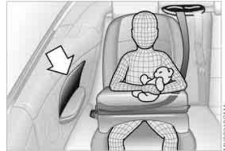
This is the right way a child should sit in a child restraint when rear side airbags are provided.
