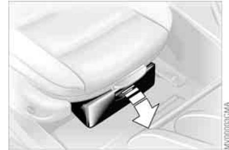
The first-aid kit is located under the front passenger's seat.
