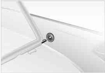
3. Hold the wind deflector so that the smaller half points toward the front and guide the mounting pin for the side piece into the proper opening
