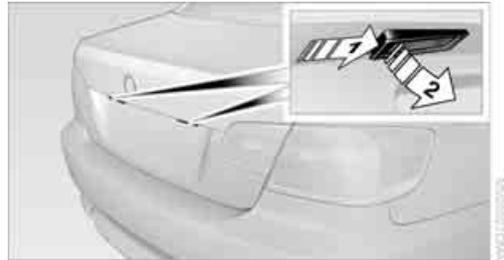
1. Using a screwdriver, push the lamp to the right in the flap of the lamp housing.
