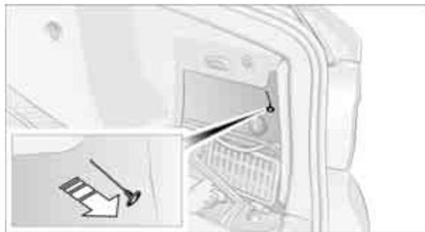
1. Remove the cover from the right-hand side-wall of the cargo bay.
