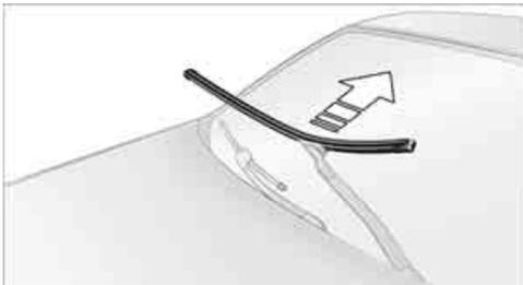
3. Fold the wiper blade upwards.
