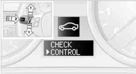
1. Push button **1** in the turn indicator stalk up or down repeatedly until the appropriate symbol appears in the display, accompanied by the words "CHECK CONTROL".
