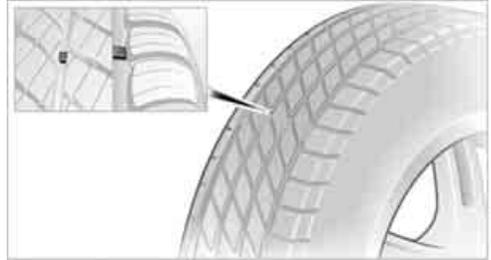
Wear indicators in the base of the tread groove are distributed around the tire's circumference; the letters TWI, for Tread Wear Indicator, on the tire's sidewalls identify tires that incorporate these wear indicators. Once the tire tread has worn down to the wear indicators, the tire has worn to a depth of 1/16 in/1.6 mm.
