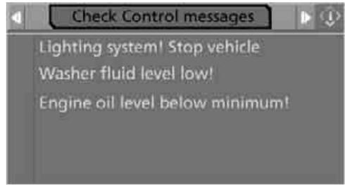
Some Check Control messages remain visible until the malfunction in question has been rectified. They cannot be hidden. If several malfunctions occur at the same time, Check Control messages are displayed in succession.
