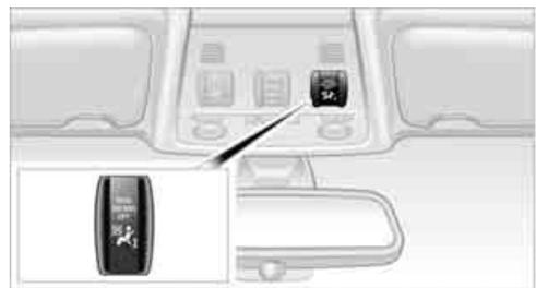
The indicator lamp for the front passenger airbags shows the functional status of the front passenger's front and side airbags in accor-
