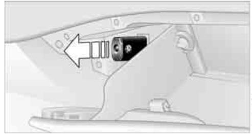
**⚠** Only insert the flashlight back into the socket when it is switched off, otherwise there is a risk of damage. ◀
