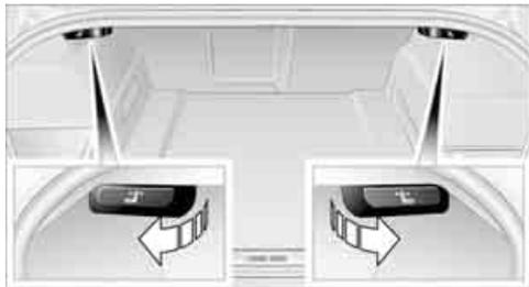
1. To release the rear seat back, pull the corresponding lever in the cargo bay.
