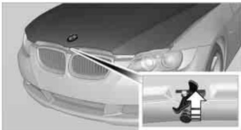
**!** In order to avoid damage, make sure that the wiper arms are against the windshield before you open the hood. ◀
