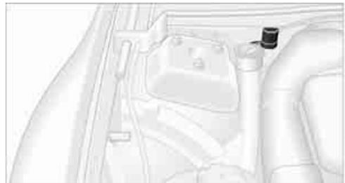
2. Attach one terminal clamp of the plus/+ jumper cable to the positive terminal of the battery or a starting-aid terminal of the vehicle providing assistance.
