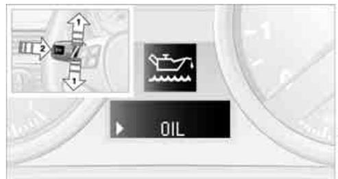
1. Push button 1 in the turn indicator stalk up or down repeatedly until the appropriate symbol is shown in the display, accompanied by the word "OIL".
