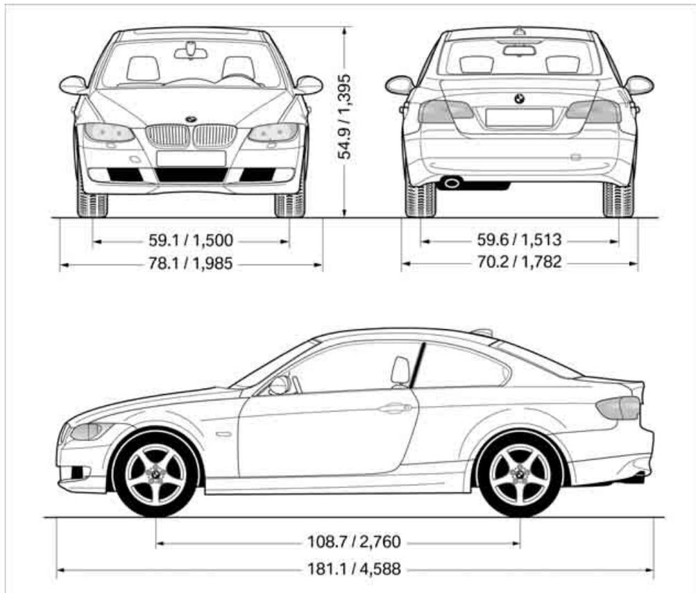
All dimensions given in inches/mm. Smallest turning circle diam.: 36 ft 1 in/11.0 m
