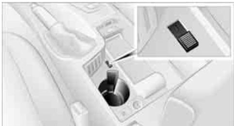
The storage compartment in the center armrest can be ventilated: slide the switch backwards.
