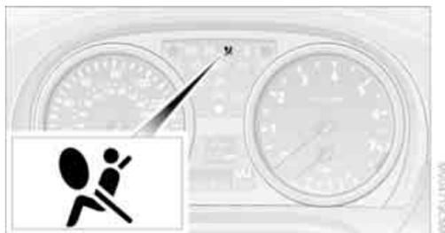
After the remote control is inserted in the ignition lock, or turned to radio-ready position, refer to page 52, the warning lamp lights up for a brief time, indicating the operational readiness of the entire airbag system and safety belt tensioners.
