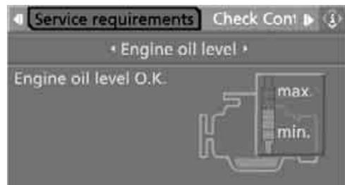
5. If necessary, move the highlight marker to the second field from the top. Turn the controller until "Engine oil level" is selected and press the controller. The oil level is displayed.
