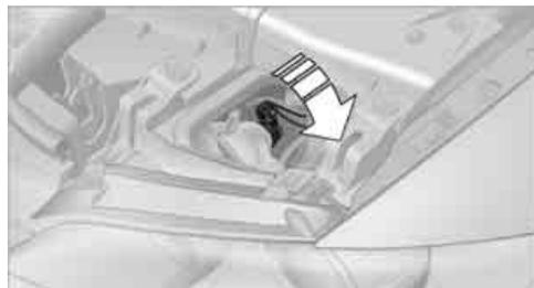
3. Disconnect the plug, change the bulb and reconnect the plug.
