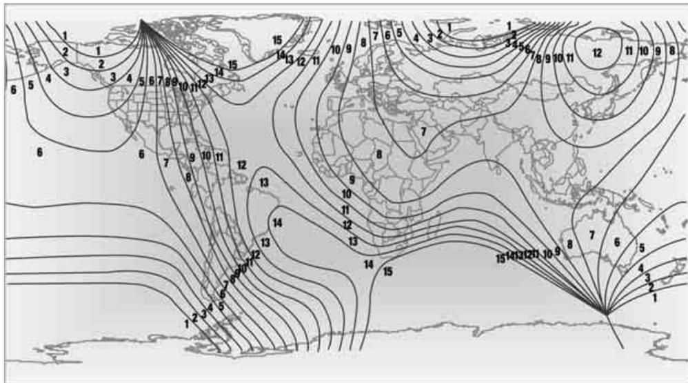
To set a compass zone, press the adjustment button on the bottom of the interior rearview mirror with a pointed object, such as a pen, for approx. 3–4 seconds. The number of the compass zone set is shown in the display.
