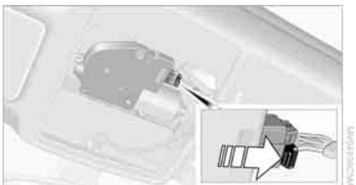
5. Insert the Allen wrench supplied with the onboard tool kit, refer to page 198, into the opening provided. Move the glass sunroof in the desired direction.
