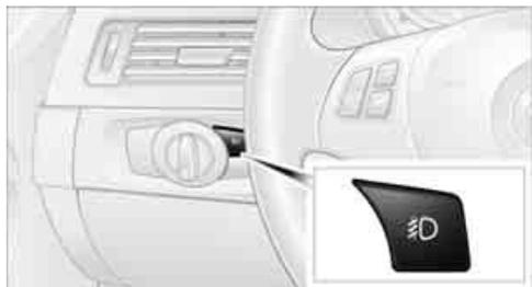
**F** The parking lamps or low beams must be switched on for the fog lamps to operate. The green indicator lamp in the instrument cluster lights up whenever the fog lamps are on.
