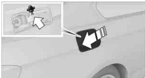
1. Open fuel filler door. To do so, lightly press the rear edge.
