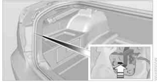
3. Turn signal indicator: apply gentle pressure to the bulb while turning it to the left for removal and replacement.
