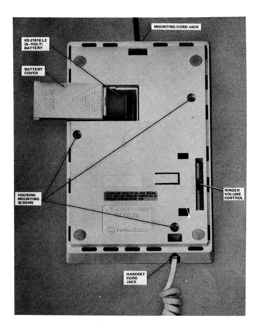
Fig. 3—5001T01A Telephone Set, Bottom View
