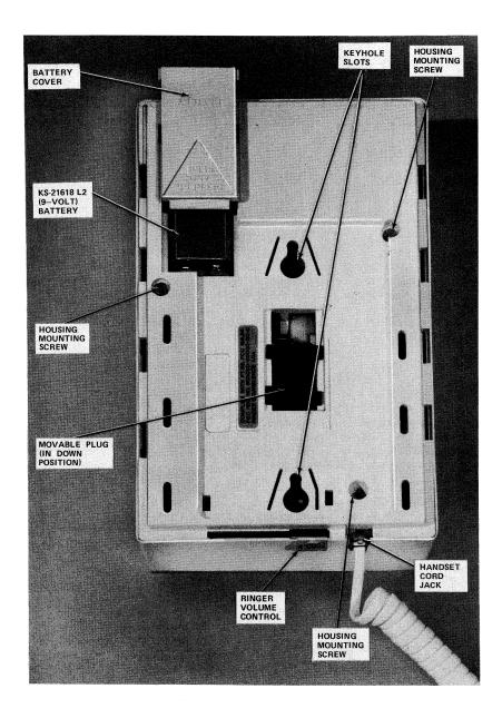
Fig. 3-5011T01A Telephone Set, Bottom View
