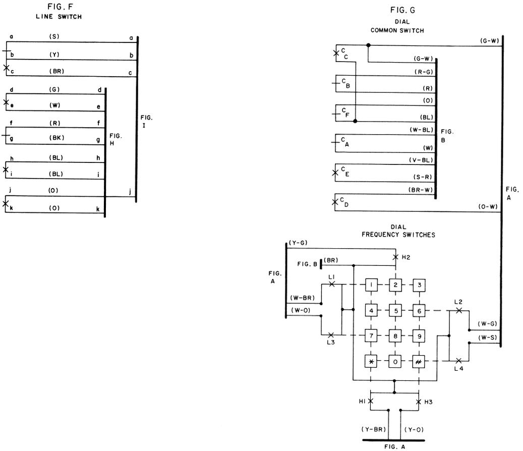
Fig. 9—2872A1M (MD) or 2872A2M Telephone Set, Connections (Sheet 3 of 5)
