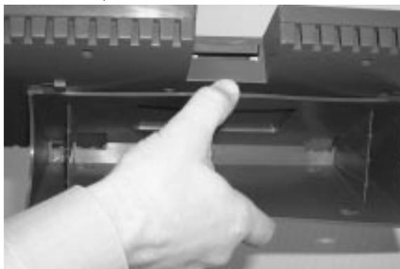
2. While applying downward pressure, simultaneously slide the bracket in the direction of the power cord.
