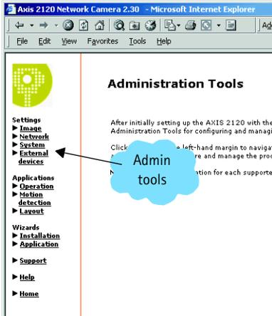
1. From the Admin tools, click **External Devices**. Select the AXIS 2191 Audio Module as the device to use. Click **Save**. **Note:** If you do not see External Devices, then your camera does not have the correct firmware installed and it must be upgraded.
