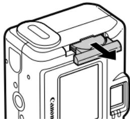
**3** Shift the date battery slightly in the direction of the arrow ① and pull out the battery in the direction as shown with arrow ②.
