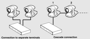
• When VC-C4/VC-C4Rs are cascade connected, ID numbers in ascending order from 1 are assigned to each camera starting with the first camera connected to camera control connectors CC1 and CC2. Cameras can be connected to Video inputs in any desired combination.
