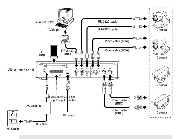
The cable connecting the VB101 and the camera should be no longer than 15 meters (49 ft. 2 <sup>19</sup>/<sub>32</sub> in.), as stipulated in the RS-232C standards. If the cable length exceeds 15 meters (49 ft. 2 <sup>19</sup>/<sub>32</sub> in.), system operation is no longer guaranteed.
