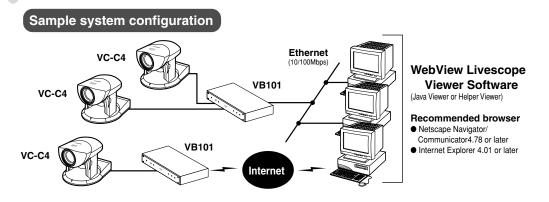
This system configuration consists of the VB101 with WebView Livescope Viewer Software ( $\rightarrow$  P.18). The WebView Livescope Viewer Software consists of the Helper Viewer and the Java Viewer.
