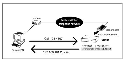
This example shows the VB101 connected in a dialup environment. In this configuration, videos can be accessed by viewers which can dial up to the VB101 using a modem.
