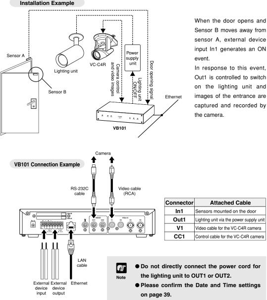
Sensor B moves away from sensor A, external device input In1 generates an ON
