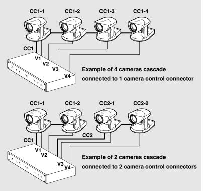
In cascade connections, if an abnormality occurs with the first camera in the connection, control for all other cameras in the cascade may not work normally.
