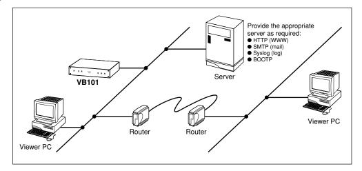
This example shows the VB101 connected to a LAN by Ethernet. In this configuration, videos can be seen by viewers in the same Ethernet segment as the VB101 and by viewers with access to that segment.
