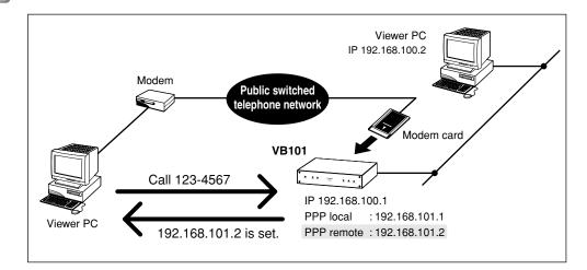
This example shows the VB101 connected to a LAN and a dial up environment. Videos can be seen by viewers in the same Ethernet segment as the VB101, viewers who can access the segment, or by viewers which can dial up to the VB101 with a modem.
