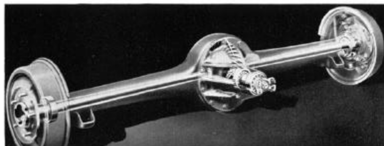
7-BEARING REAR AXLE— Seven anti-friction bearings are used in the construction of this unusually sturdy axle, insuring long life and a minimum of rolling resistance. Long-life design is employed throughout.
