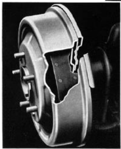
TRIPLE-SEALED BRAKES— Brakes are equipped with three-way seals which prevent dirt, mud and water from reaching the brake mechanism.
