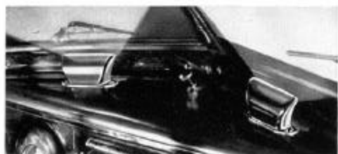
DUAL WINDSHIELD DEFROSTER —Throws two streams of warm air against inside of windshield.
