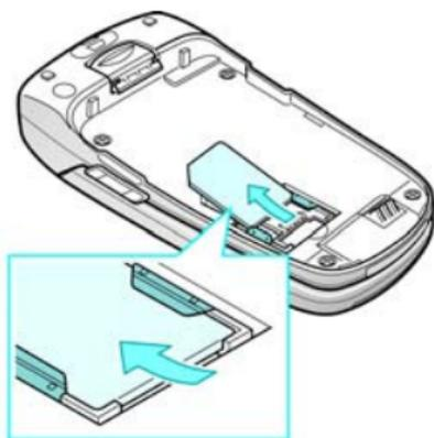
4. Place the battery back, taking care to match the tabs on the battery with the grooves on the phone.
