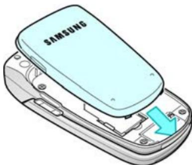
5. Press the battery down until it clicks into place. Make sure that the battery is properly installed before switching on the power.
